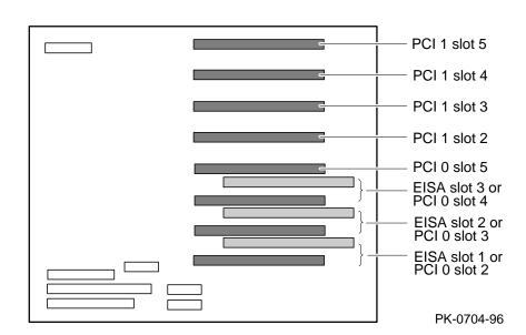
Figure 1-9 PCI Motherboard (PCI 0 and 1)
