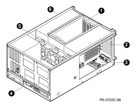
The callouts in Figure 1–3 point to these components of the BA30B system drawer:
