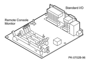
The server control module has two sections: the remote console monitor and the standard I/O connectors.
