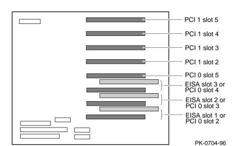
Figure 4-9 PCI and EISA Slots (PCI 0 and 1)
