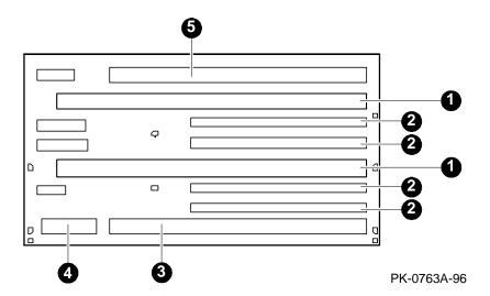
The system motherboard has the logic for the system bus. It is the backplane that holds the CPU, memory, bridge, and power control modules. Figure 1–4 shows the locations of these modules and of connectors on the motherboard.
