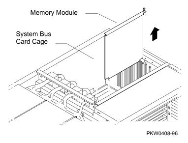
WARNING: CPU modules and memory modules have parts that operate at high temperatures. Wait 2 minutes after power is removed before touching any module.
