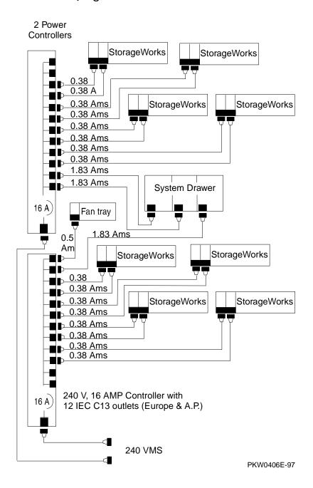
Figure 4-8 -EL Three Drawer Cabinet Power Configuration (Three drawer -EL shown with H7600-AA controller)
