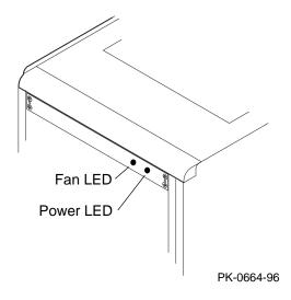
A cabinet system has three exhaust fans at the top of the cabinet. They are powered from a small power supply in the fan tray. This power supply also powers the server control module at the bottom of the PCI card cage to allow remote access to the system. A failure of the power supply is indicated only by the LEDs. No messages are displayed.
