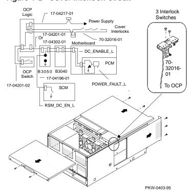
*NOTE:* The cover interlocks must be engaged to enable power-up.
