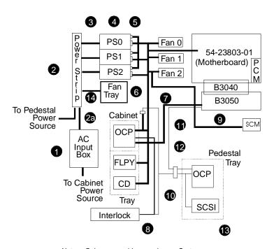
Notes: Only power cables are shown. Systems have only one OCP located in either the cabinet tray or the pedestal tray. Thicker lines indicate cables present in both cabinets. Thinner lines are cables in the pedestal only. PKW-0401a-96
