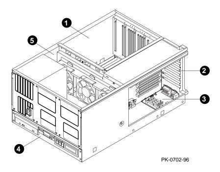
When the system drawer is in a pedestal, the control panel assembly is mounted in a tray at the top of the drawer.
