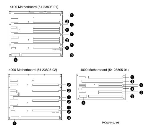
The system motherboard has the logic for the system bus. It is the backplane that holds the CPU, memory, bridge, and power control modules. Figure 1-13 shows diagrams of the three motherboards used in AlphaServer 4000/4100 systems. The module locations are designated by the callouts.
