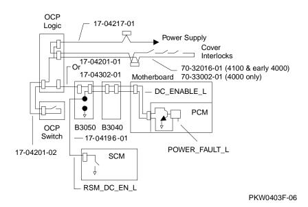
Figure 4-3 shows the distribution of power thoughout the system drawer. Opens in the circuit or the PCM signal POWER\_FAULT\_L or the SCM signal RSM\_DC\_EN\_L interrupt DC power applied to the system. The opens can be caused by the On/Off button or the cover interlocks. The POWER\_FAULT\_L signal is asserted by the PCM module if it detects a fault and the RSM\_DC\_EN\_L is controlled remotely.
