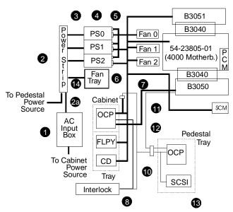
Note: Only power cables are shown. Systems have only one OCP located in either the cabinet tray or the pedestal tray. Thicker lines indicate cables present in both cabinets. Thinner lines are cables in the pedestal only. Callout is intentionally missing.
