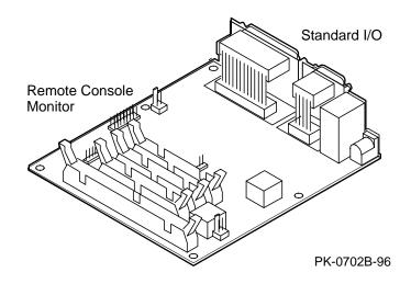
The server control module has two sections: the remote console monitor (RCM) and the standard I/O. See Appendix C for information on controlling the system remotely.
