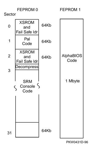
For the console to run, the path from the CPU to the XSROM must be functional. The XSROM resides in FEPROM0 on the XBUS, off the EISA bus, off PCI 0, off IOD 0. See Figure 2-4. This path is minimally tested by SROM.
