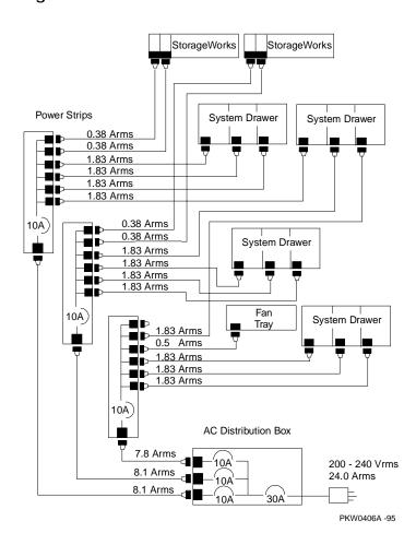
Figure 4-6 Worst-Case -EB & -EC Cabinet Power Configuration
