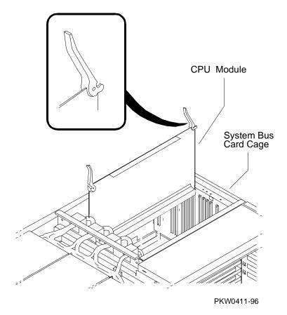
WARNING: CPU modules and memory modules have parts that operate at high temperatures. Wait 2 minutes after power is removed before touching any module.
