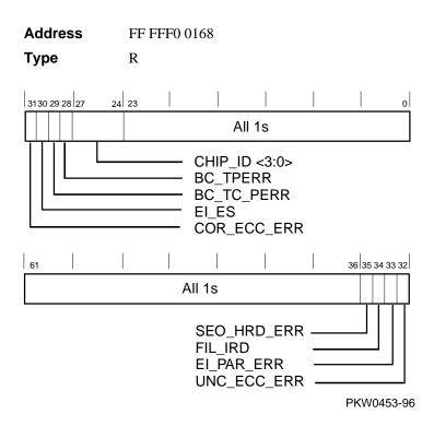
Fill data from B-cache or main memory could have correctable or uncorrectable errors in ECC mode. In parity mode, fill data parity errors are treated as uncorrectable hard errors. System address/command parity errors are always treated as uncorrectable hard errors, irrespective of the mode. The sequence for reading, unlocking, and clearing EI\_STAT, EI\_ADDR, BC\_TAG\_ADDR, and FILL\_SYN is as follows:
