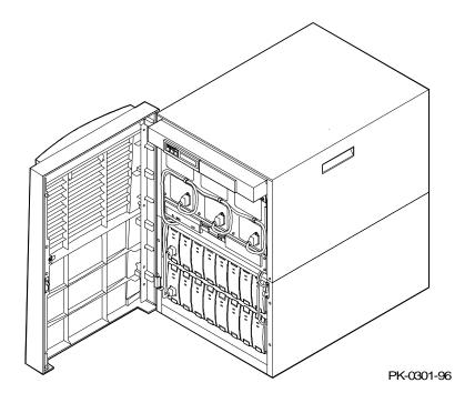
In the pedestal system, the control panel is located at the top left in a tray. See Figure 1-11. There is space for an optional device beside it.
