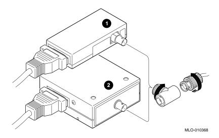
Step 5: Terminate Connection If your workstation is the last one on a ThinWire network, you need to terminate the network connection. Do this by connecting a terminator, rather than a ThinWire network cable, to one side of the T-connector on the DECXM transceiver ①, or a DESTA unit ②, as shown in Figure 4–5.
