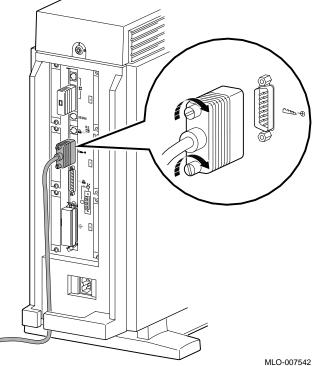
Step 3: Connect the Keyboard Cable and Mouse Cables Connect the keyboard cable and the mouse cable to the connector block on the keyboard/mouse extension cable ①, as shown in Figure 3–4. The extension cable is provided so that the mouse and keyboard can be located away from the system unit.
