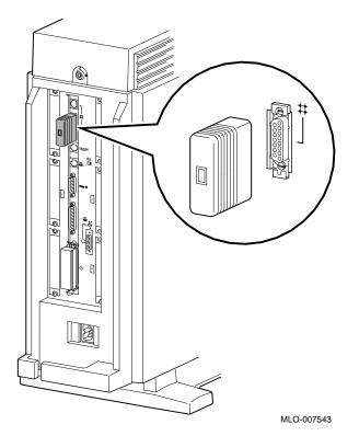
Step 2:<br/>Connect the<br/>Keyboard/Mouse<br/>Extension<br/>CableConnect the keyboard/mouse extension cable to the keyboard/<br/>mouse port on the system unit, as shown in Figure 3–3.Figure 3–3<br/>Connecting the Keyboard/Mouse Extension Cable
