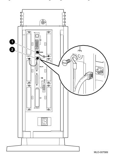
Figure C–1 Connecting a Pigtail Grounding Wire
