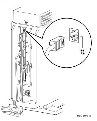
Figure 4–2 Connecting a 10BASE-T Network Cable
