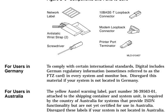
Figure 2–6 Components and Parts to Save
