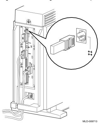
Figure 13–8 Connecting the 10BASE-T Loopback Connector
