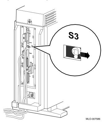
Figure 3–10 Checking the Alternate Console Switch
