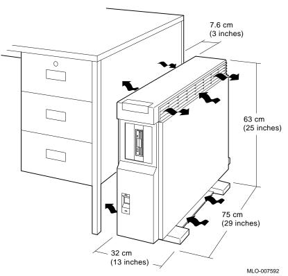
Monitor Requirements When allocating space for your new DEC 3000 Model 500X AXP workstation, consider also the size of your monitor and the length of your monitor video cable.
