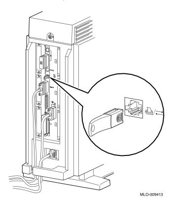
Modem Loopback Connector If your Digital service representative requests that you connect the modem loopback connector, connect it as shown in Figure 13–10.
