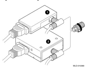
Figure 4–5 Terminating the Ethernet Connection
