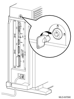
Figure 3–12 Locking the System Unit Cover
