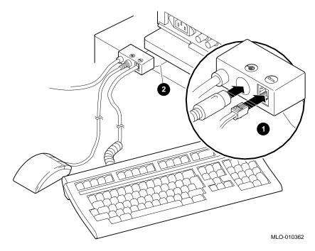
The Plastic Mylar Tab To keep the keyboard/mouse extension cable in one location, you can place the plastic Mylar tab ② on the connector block of the keyboard/mouse extension cable under the base of your monitor.
