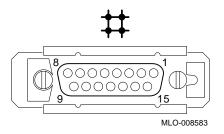
AUI Ethernet Port Pin-outs Table B-5 describes pin usage for the AUI Ethernet port.
