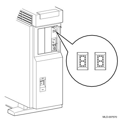
The diagnostic display lights can provide your Digital service representative with important information in determining the source of a problem.
