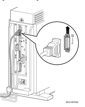
Figure 4–1 Connecting to an AUI Ethernet Network
