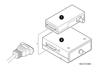
Step 4: ThinWire Cables and T-Connector Connect the ThinWire network cables to the T-Connector and then the T-connector to the DECXM transceiver **①**, or a DESTA unit **②** unit, as shown in Figure 4–4.
