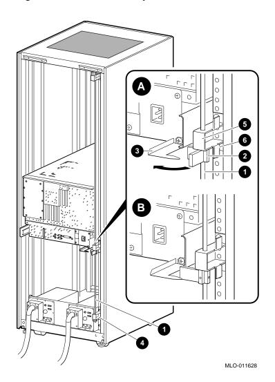
Figure 2–11 The Interlock System
