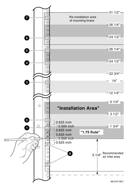
Figure 2–12 Vertical Mount System: Installation Area English (RETMA)
