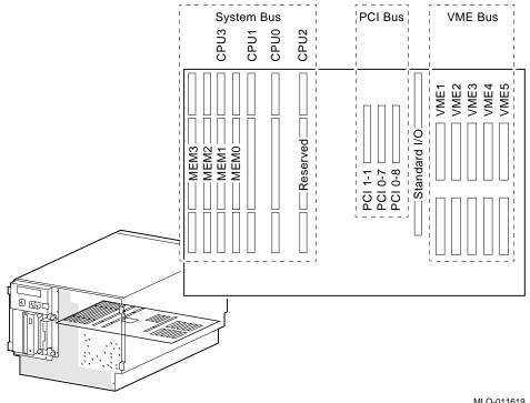
Figure 5–3 Drawer Mount System: Bus Option Locations
