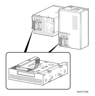
Figure 5–7 Attaching the Tape Drive Insulator Strip
