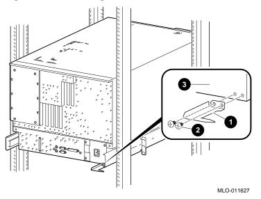
Figure 2–10 Installing the Interlock Actuator Bracket
