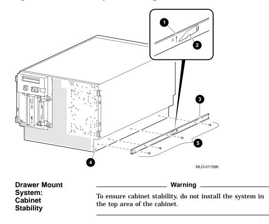
Figure 2–4 Drawer Mount System: Attaching the Slide Races
