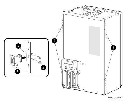
Figure 2–14 Vertical Mount System: Attaching the Four Bezel Tabs
