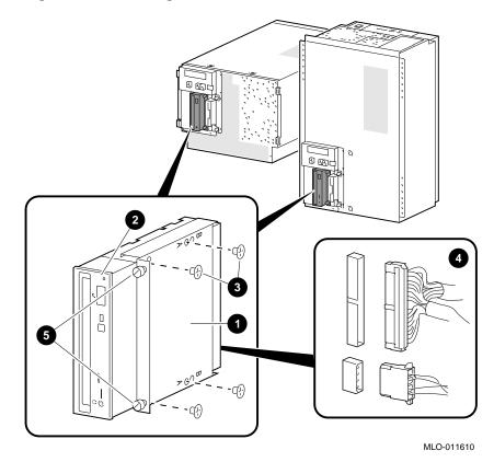
Figure 5–8 Installing Removable Media
