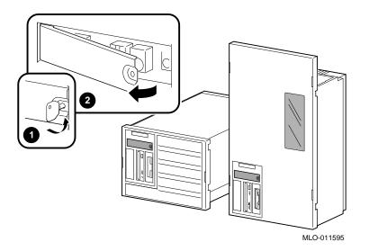
Drawer Mount System: Top Access Cover Figure 1-6 shows the location of the top access cover to the module card-cage area.
