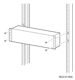
Vertical Mount System: Installing the System To install the system, perform the following steps:
