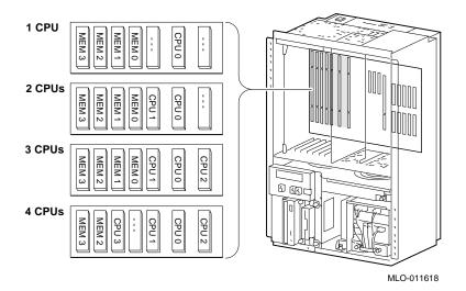
Figure 5–4 Vertical Mount System: System Bus Configurations
