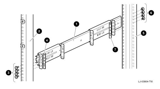
Drawer Mount System: Mounting the System on the Slides To mount the system on the slides, refer to Figure 2–8 and proceed as follows:
