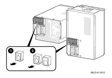
Figure 2–23 Turning Off the System
