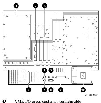
Figure 1–9 shows the bulkhead components (top of the system).
