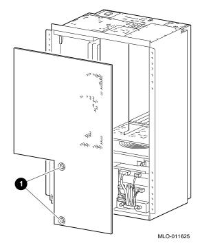
Figure 1–7 Vertical Mount System: Front Access Cover
