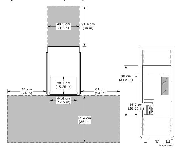
Figure 2–2 Vertical Mount System: System Clearance/Service Area
