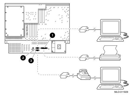
Figure 2–26 Connecting Serial and Parallel Devices
