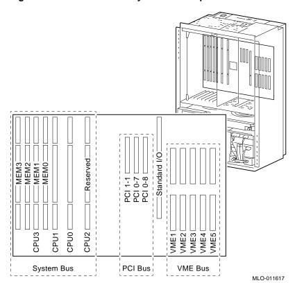
Figure 5–2 Vertical Mount System: Bus Option Locations
