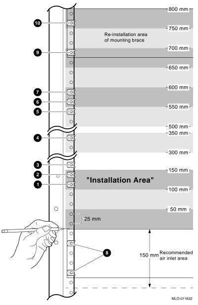
Figure 2–13 Vertical Mount System: Installation Area Metric (IEC)
