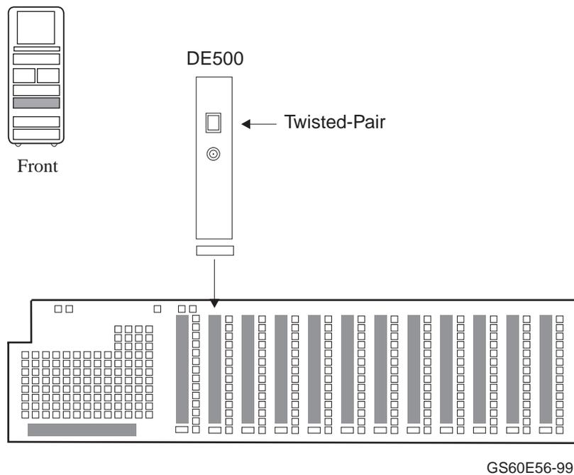
The DE500, the PCI Ethernet adapter, implements the twisted-pair Ethernet variant.
