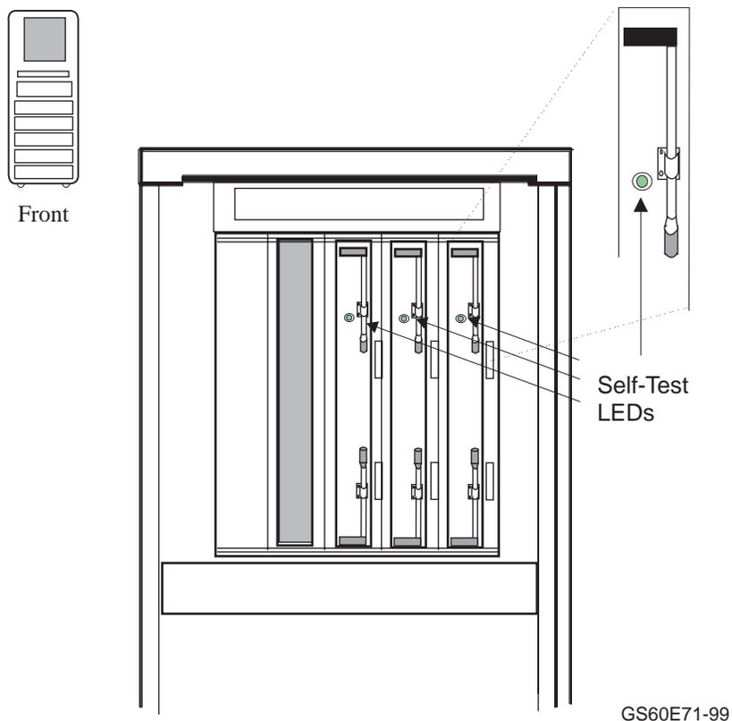
Processor and memory modules have a green LED that lights when the module passes or completes self-test. These LEDs can be viewed through holes in the shield of the module enclosure from the front of the cabinet. PCI I/O modules are not visible but some connectors have LEDs on them. Table 6-1 lists TLSB and DWLPB, the PCI motherboard, modules showing LED conditions after self-test. For conditions of LEDs on PCI adapters, see the related documentation.
