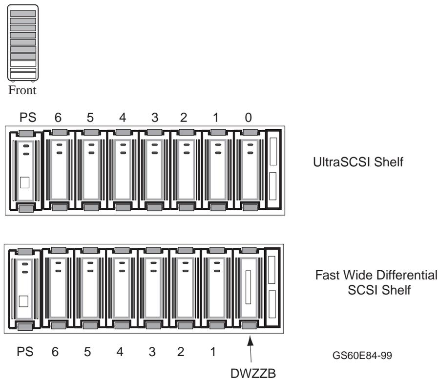
Check the output from the **show device** command against the physical SBBs. There should be a one-to-one correspondence between SBBs reporting to the console and the physical devices mounted. Note that the node number reported by the console corresponds to the physical position of an SBB within a shelf; the slots and nodes are numbered 0 to 6, from right to left (see Figure 8-4).
