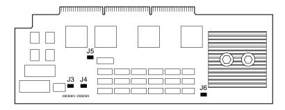
Figure 1-2. CPU Module Jumper Locations
