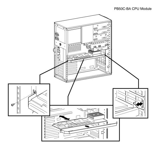
Figure 1-3. Installing the PB50C-BA CPU Module
