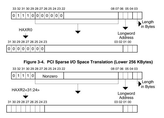
Figure 3-5. PCI Sparse I/O Address Translation (Remaining 16 MBytes)
