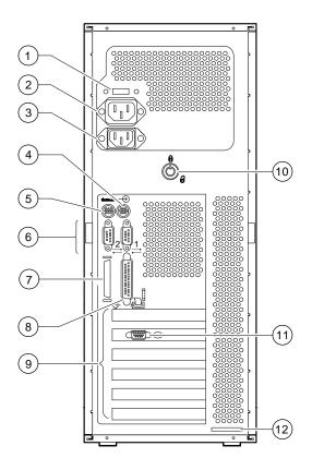
Figure 1-4. AlphaStation 400 Series Rear Connectors
