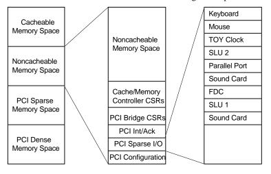
Figure 3-6 shows some of the devices that are accessed through PCI sparse address space.
