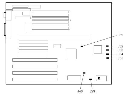
Figure 2-6. AlphaStation 400 Series Motherboard Jumpers
