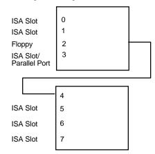
Figure 5-1. DMA Channel Assignments
