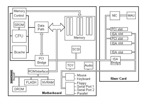
Figure 1-5. AlphaStation 200 Series System Architecture
