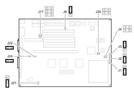
Figure 2-4. AlphaStation 200 Series System Motherboard Jumpers
