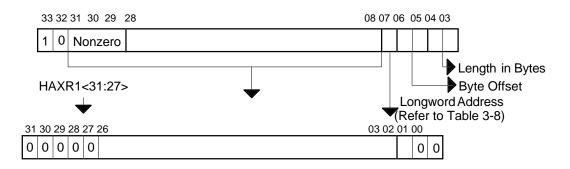
Figure 3-9. PCI Memory Space Address Translation (Remaining 112 MBytes)
