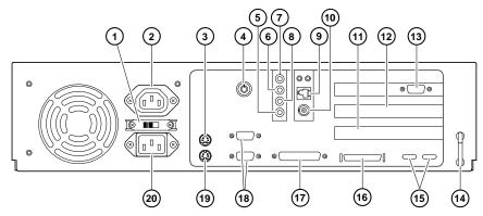
Figure 10-1. AlphaStation 200 Series System Rear Connectors
