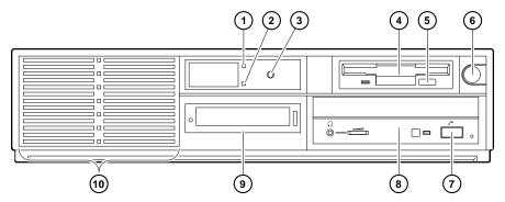
Figure 1-1. AlphaStation 200 Series Control and Indicators
