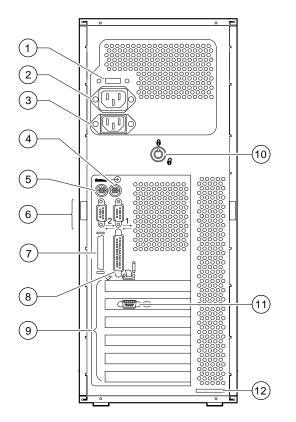
Figure 10-2. AlphaStation 400 Series System Rear Connectors
