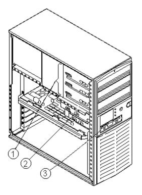
Figure 2-2. Internal Bays - AlphaStation 400 Series Systems
