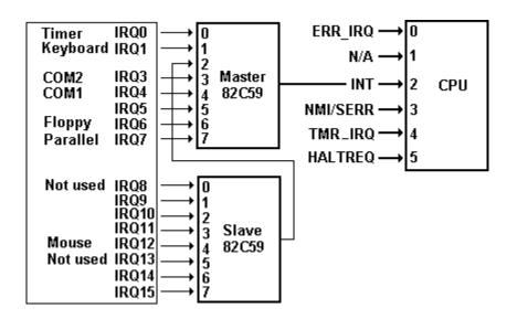
Figure 6-1. Interrupt System Block Diagram
