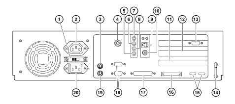
Figure 1-2. AlphaStation 200 Series Rear Connectors
