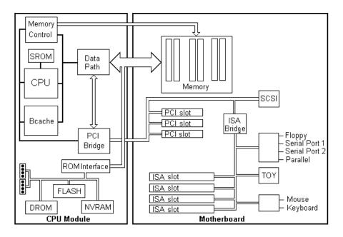
Figure 1-6. AlphaStation 400 Series System Architecture
