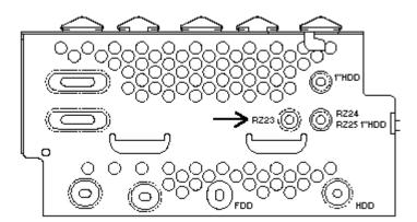
3. Use two screws to mount the drive to the drive bracket, as shown below.
