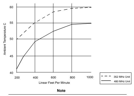
The maximum temperature, when measured between the heat sink studs on the base of the heat sink, must be less than  $68^{\circ}$  C.
