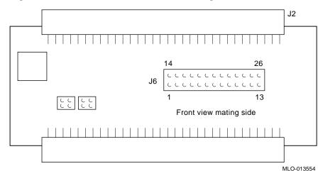
Figure C–6 Parallel Port Connector Pin Assignments
