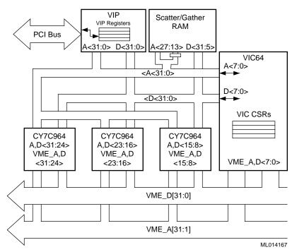
Figure 3–4 PCI-to-VME Interface Components
