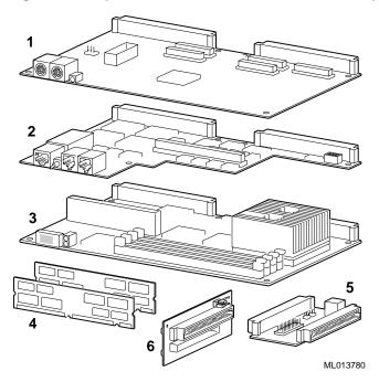
Figure 2–1 Alpha VME 5/352 and 5/480 Module Components
