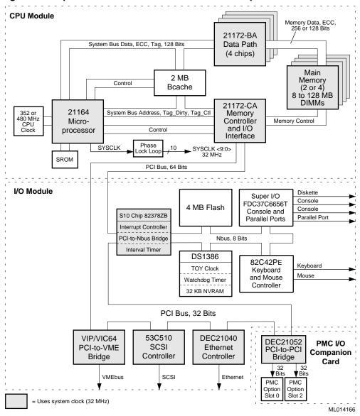
Figure 3–1 Alpha VME 5/352 and 5/480 Functional Components
