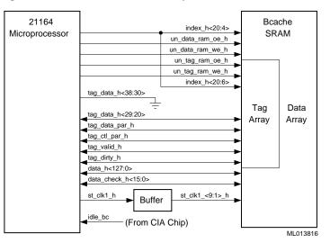
Figure 3–3 Level 3 Bcache Array
