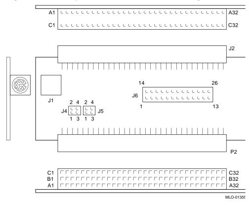
Figure C-4 Secondary Breakout Module Connector Pin Assignments
