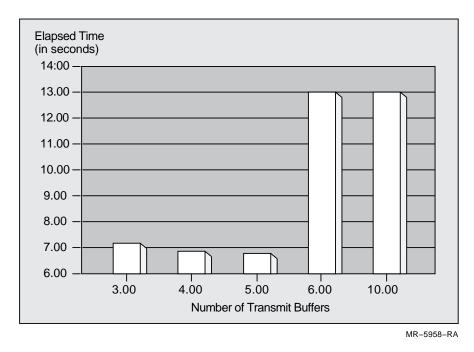
Figure 3–1 DECnet 1-Megabyte File Transfer with a Third-Party Ethernet Board
