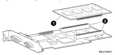
Orient the RAM expansion module **①** so that its connectors align with those on the graphics module. Note that one of the connectors on the expansion module has a missing pin and aligns with a corresponding connector on the graphics module. Attach the expansion module as shown in Figure 1.
