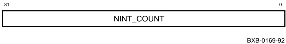
Figure 1-22 ICR — Interval Count Register
