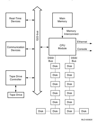
Figure 1–1: VAX 4000 Model 300 Block Diagram
