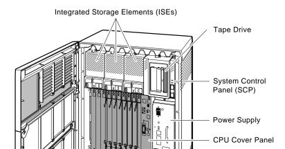
Figure 1-5: Front View of the BA430 Enclosure
