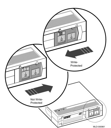
Figure 3-10: Tape Cartridge Write-Protect Switch
