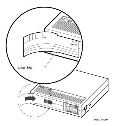
**NOTE:** Do not write on the tape cartridge or attach labels to the top, bottom, or sides of the cartridge.
