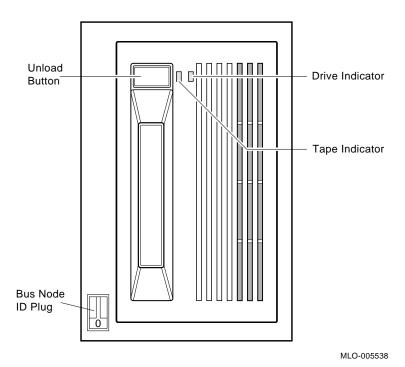
The Unload button is used to eject the cassette tape. The Tape and Drive indicators show the status of the TLZ04 and can indicate possible error conditions.
