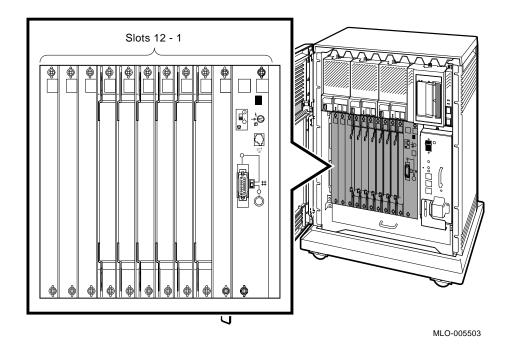
The first slot is reserved for the central processing unit (CPU). Up to four MS650 memory modules may follow the CPU. The CPU and the first memory module (slots 1 and 2) are covered by a dual-width CPU cover panel with system controls and connectors. The remaining slots are available for Q-bus option modules.
