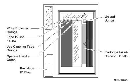
To operate the drive properly, you must carefully monitor the indicators. The instructions for inserting and removing cartridges, which appear later in this section, tell you what should happen at each step. A table at the end of the section summarizes indicator and control combinations.
