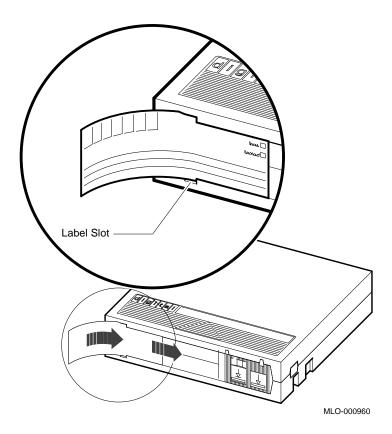
To indicate that the tape was recorded on a TK70 tape drive, check the box labeled 296MB. The 95MB box is used for tapes recorded on a TK50 drive.
