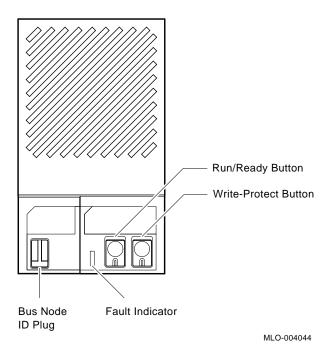
Each ISE has the following controls and indicators on its front panel:
