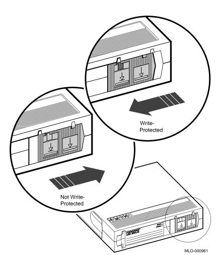
Figure 3-5: Tape Cartridge Write-Protect Switch
