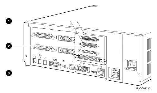
Figure 1–2 VAX 4000 Model 100 Expansion Ports
