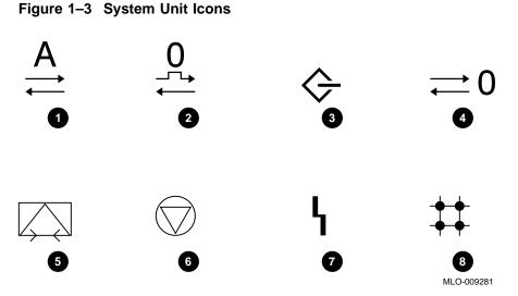
• This icon indicates optional asynchronous communications port A. A similar icon indicates the optional asynchronous communications port B.
