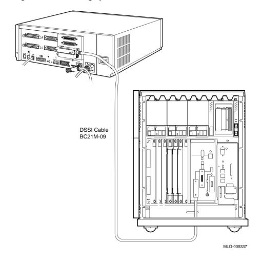
Figure 3–9 Connecting Systems Into a VAXcluster
