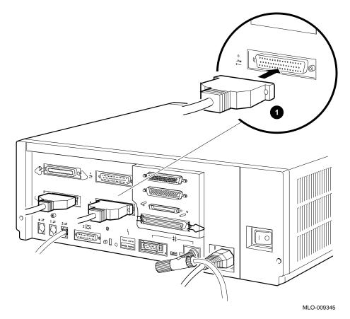
Figure 4–8 Connecting the Cable to Synchronous Port 0
