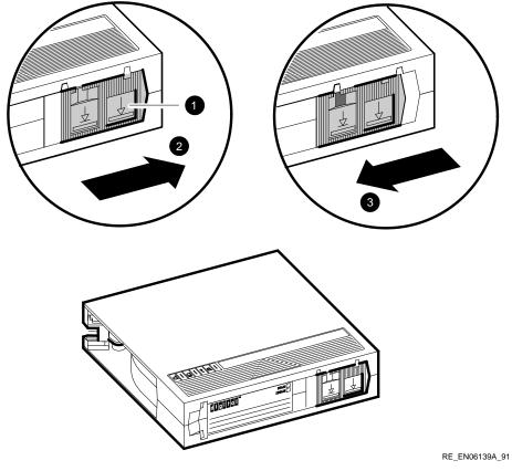
Figure B–3 Write-Protect Switch Positions
