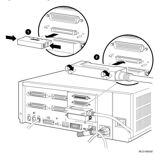
Figure 3–8 Connecting a DSSI Cable
