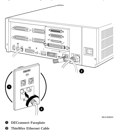
Figure 3–4 Connecting the System Unit to a DECconnect Faceplate
