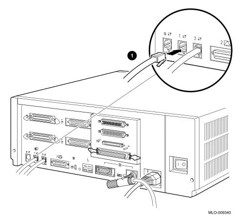
Figure 4–3 Connecting a Peripheral to MMJ Port 1
