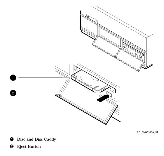
If the eject button is disabled by software, you must manually remove the caddy.
