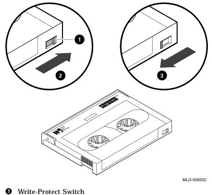
Figure B–7 Setting the Write-Protect Switch on the TLZ04 Cassette Tape
