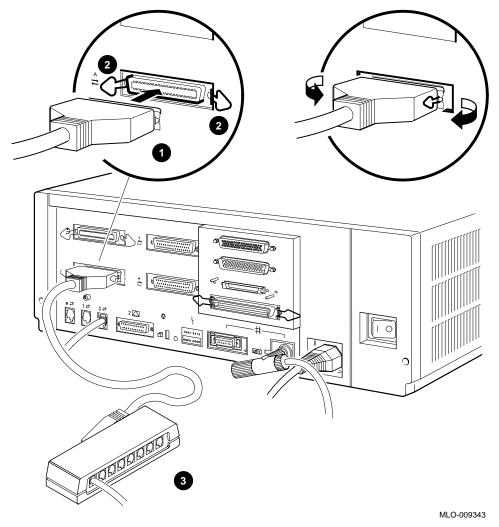
Figure 4–6 Connecting a Peripheral to Asynchronous Port A
