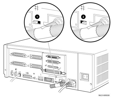
Figure 3–1 Network Select Switch Positions
