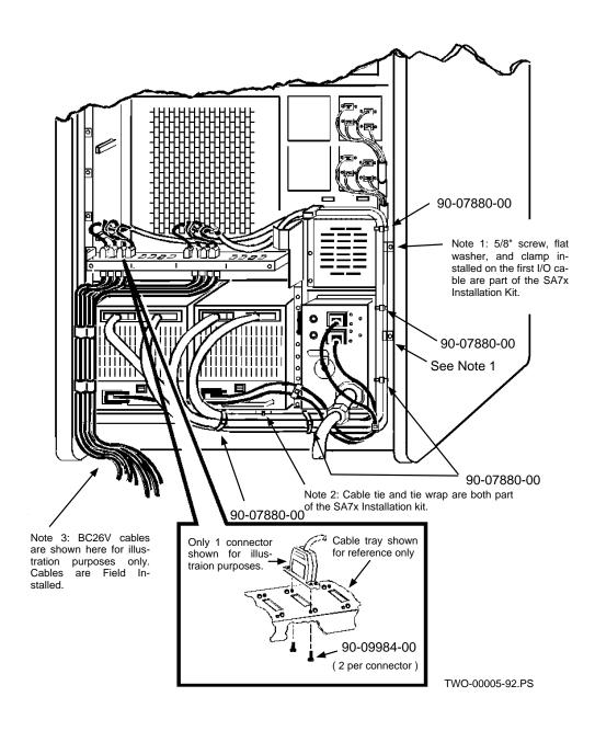
Figure 4-4: Single SA7x...A and B Ported to a HSC
