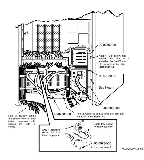
Figure 4-6: Single RA9x...A Ported to KDB50...B Ported to a HSC
