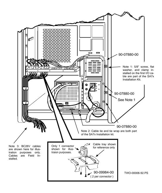
Figure 4-5: Dual SA7xs...A and B Ported to a HSC
