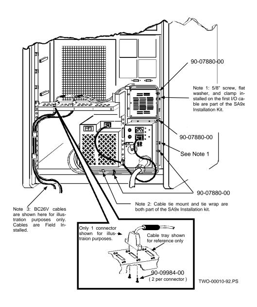
Figure 4-9: Dual RA9xs...A and B Ported to a HSC
