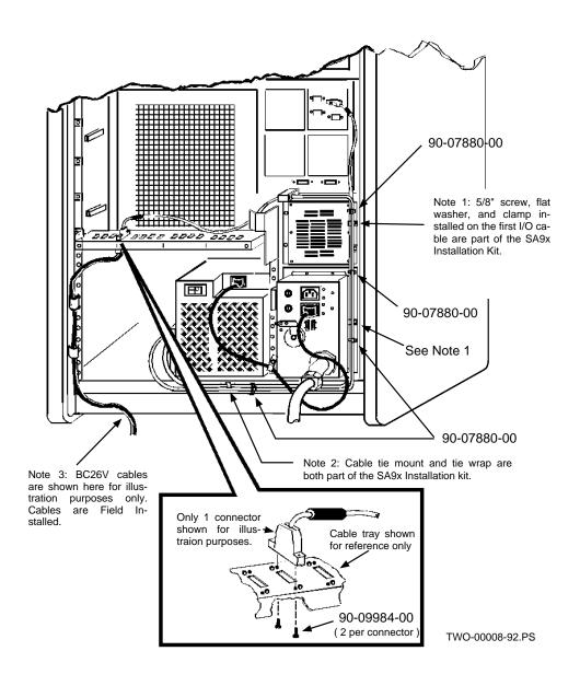
Figure 4-7: Dual RA9xs...A Ported to KDB50...B Ported to a HSC
