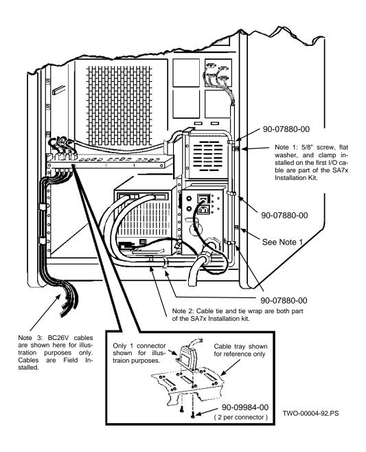
Figure 4-3: Dual SA7xs...A Ported to KDB50...B Ported to a HSC
