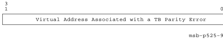
Figure 4–40: TB Parity Address Register (TBADR) IPR236 (EC)
