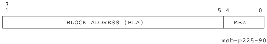
Figure 5–17: EEPROM Control Register (EECTL) BB + 70
