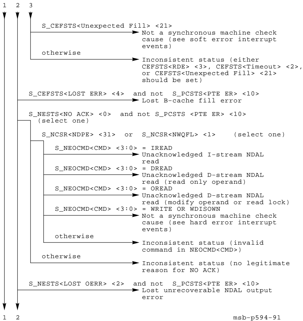
Figure 4-60 (Cont.): Machine Check Parse Tree
