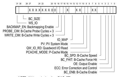
NOTE: X bits read values from DIAG\_CTL. This register reads inverted.
