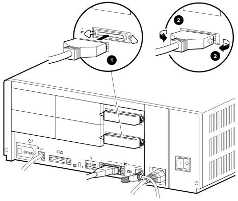
Figure 4–3 Connecting the SCSI Cable (Port A Shown)
