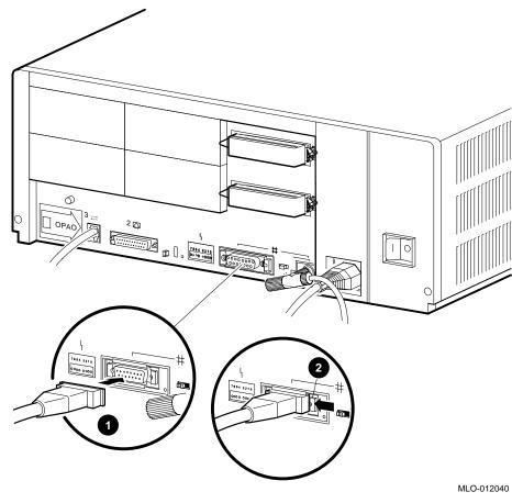
Figure 3–5 Connecting a Transceiver Cable
