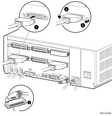
Figure 4–7 Connecting a Peripheral to Asynchronous Port A
