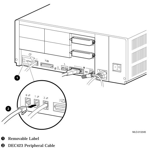
Figure 4–4 Connecting a Peripheral to MMJ Port 1
