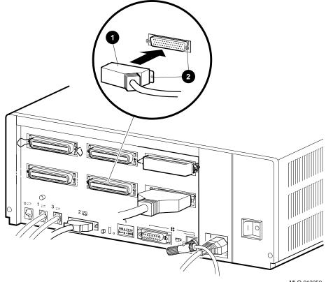
Figure 4–9 Connecting a Peripheral to Synchronous Port 0
