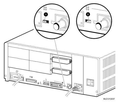
Figure 3–1 Network Select Switch Positions
