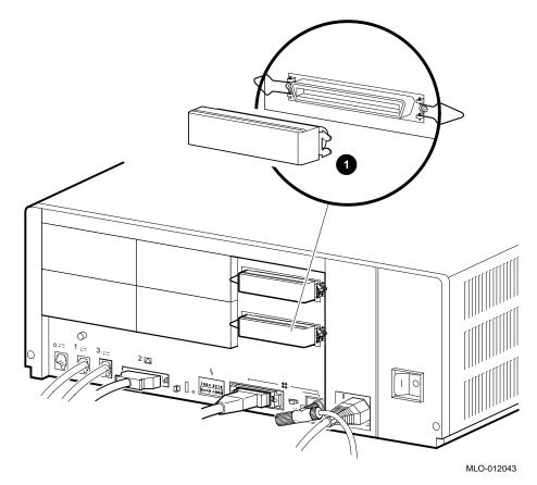
Figure 4–2 Removing the SCSI Terminator (Port A Shown)
