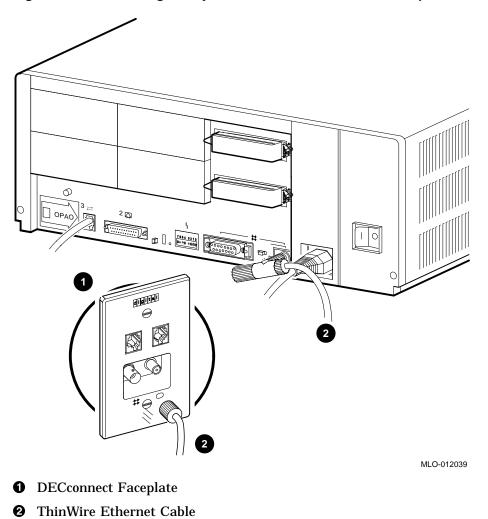
Figure 3–4 Connecting the System Unit to a DECconnect Faceplate
