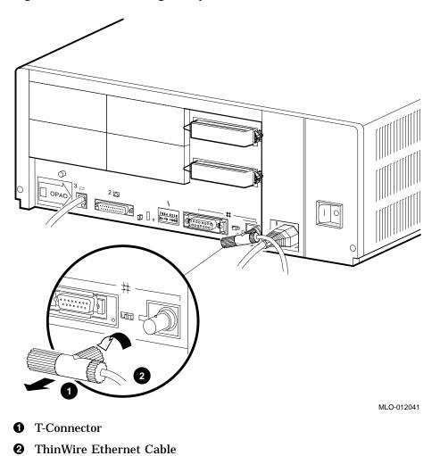
Figure 3–6 Disconnecting the System Unit from a ThinWire Ethernet Cable
