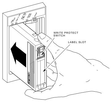
Insert a TK tape cartridge into the TF70 drive as follows:
