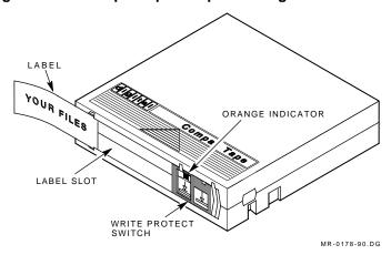
Only CompacTape II high-density cartridges should be used. They provide about 296 MB of formatted data storage.
