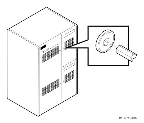
Figure 3-3 also shows the key (supplied with the system) used to turn the latch.
