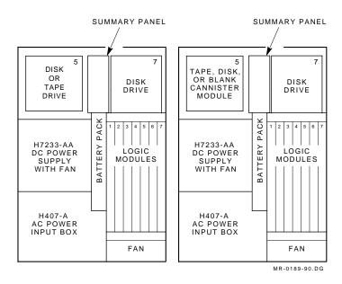
The power system for each cabinet consists of two packages: ac power input box and dc power supply. The ac power input box converts its input to unregulated dc.
