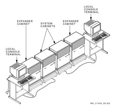
Figure 1–10 Layout of Model 310 and 410 System with Expansion
