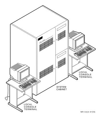
Figure 1–12 Layout of Model 610 Base System
