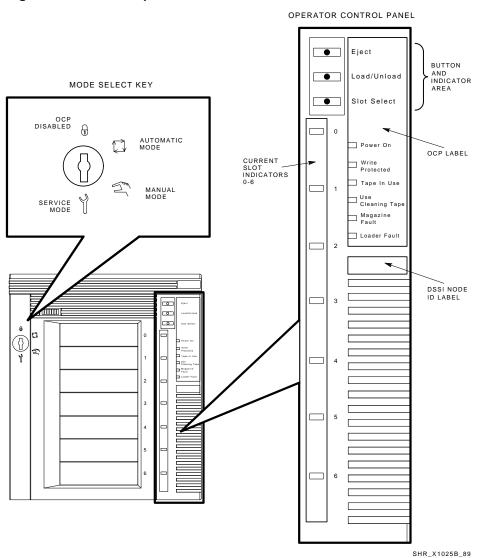
Manual mode — Automatic loading and unloading of cartridges does not occur in this mode; rather, press the Load/Unload button to move each cartridge. This mode is most useful for, but not restricted to, copying specific files to or from tape.
