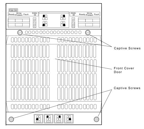
Figure 5–22 SF73 Disk Drive, Front View
