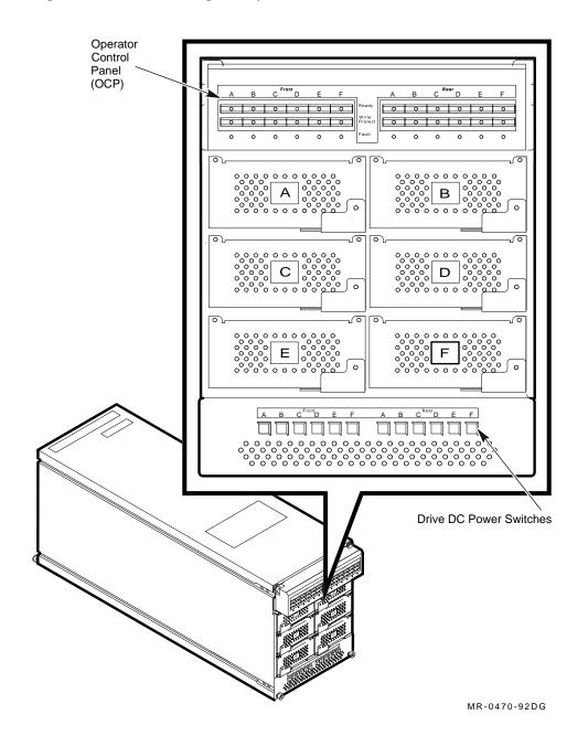
Figure 5–26 SF35 Storage Array, Front View
