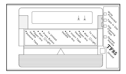
Figure 3–10 TF85C Cartridge Tape Drive
