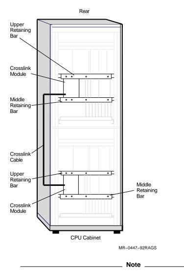
The cross-link assembly consists of two cross-link modules (one per zone) and one cross-link cable. These three parts are considered to be one FRU.
