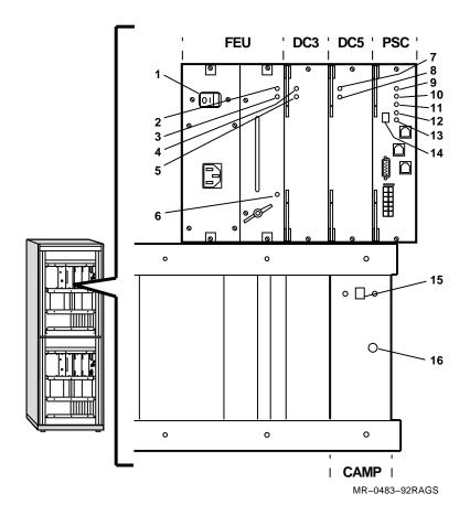
Figure 1–4 Power Module Controls and Indicators
