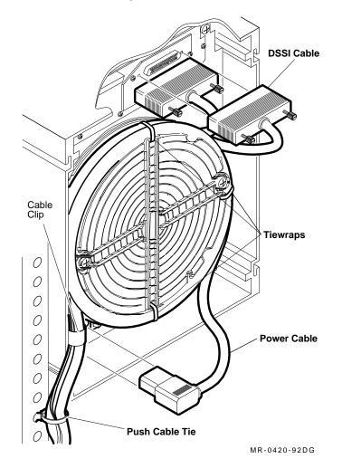
Figure 5–28 TF857-CA Tape Drive, Rear View
