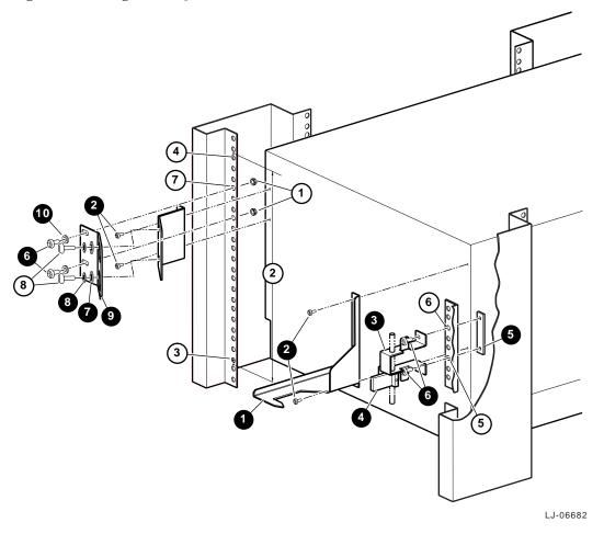
Figure 1 Installing the 2T-QINTL-55 Interlock Kit
