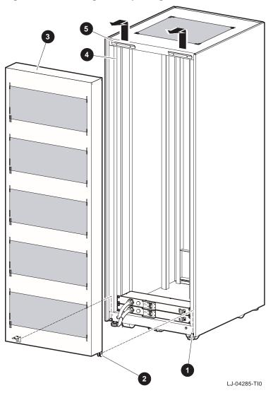
Figure 2-4 Removing and Replacing the Lift-Off Rear Door
