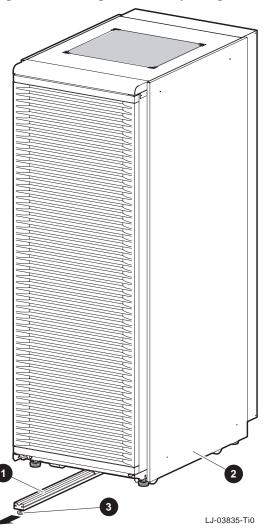
Figure 2-8 Pulling Out and Adjusting the Stabilizer Bar
