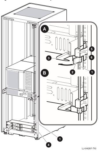
Figure 4-12 The Interlock System
