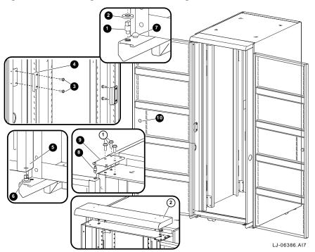
Figure 4-5 Reversing the Rear Door Swing
