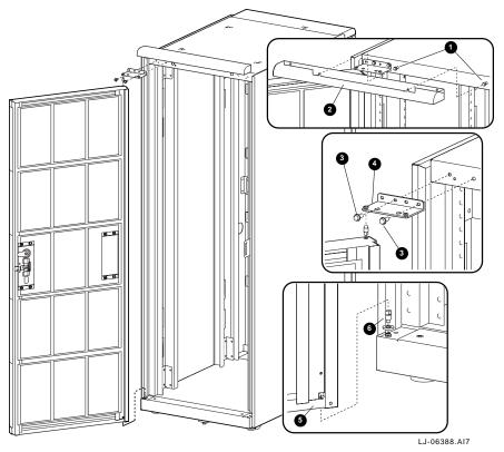
Figure 4-6 Removing and Replacing the Front Door
