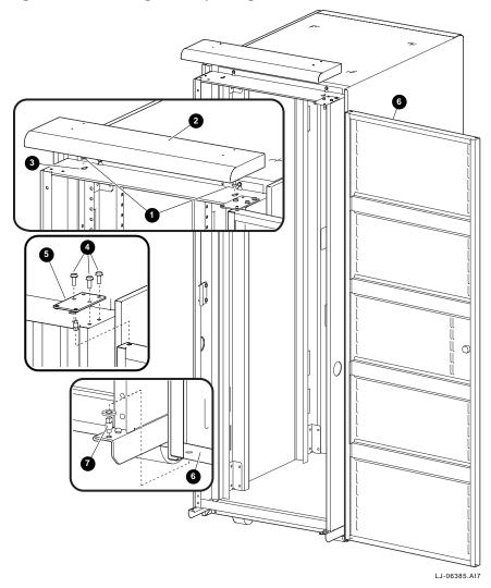
Figure 4-4 Removing and Replacing the Rear Door
