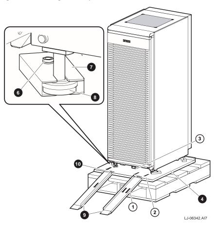
Figure 4-2 Installing the Ramps
