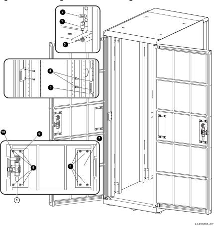
Figure 4-7 Reversing the Front Door Swing
