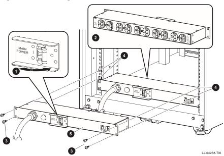
Figure 2-10 Removing a Power Distribution Unit
