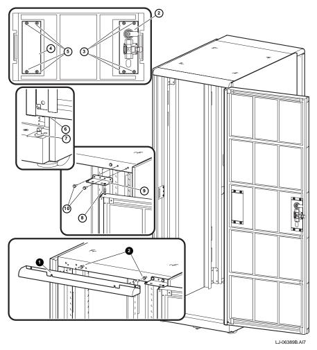
Figure 4-8 Completing the Front Door Reversal
