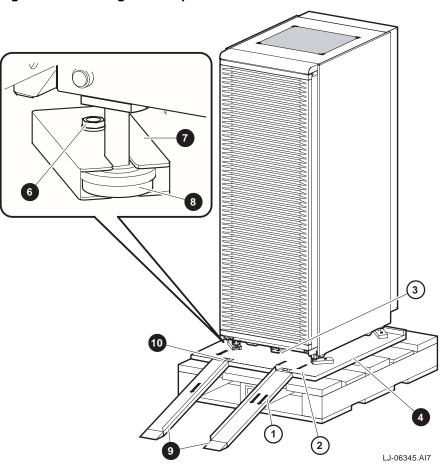
Figure 2-2 Installing the Ramps
