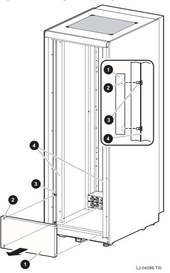
Figure 4-9 Removing and Replacing the Metal Front Filler Panels
