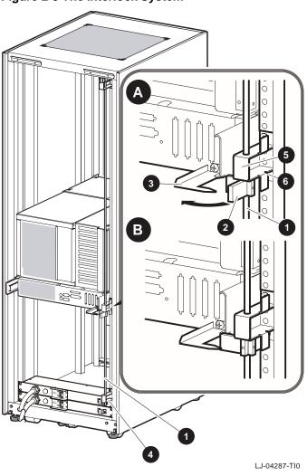
Figure 2-9 The Interlock System
