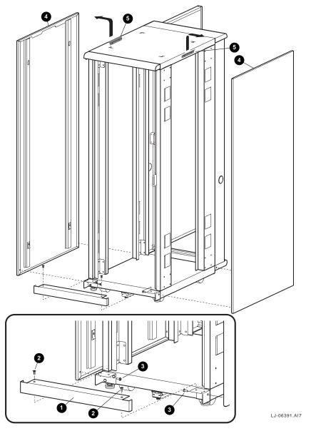
Figure 4-10 Removing and Replacing the Side Panels
