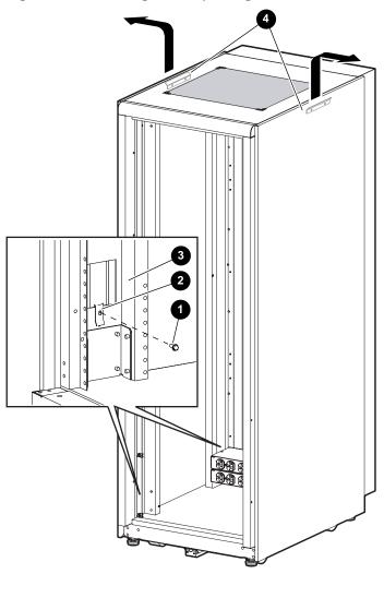
Figure 2-7 Removing and Replacing the Side Panels
