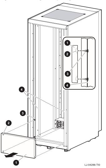
Figure 2-6 Removing and Replacing the Metal Front Filler Panels
