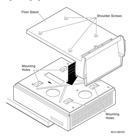
Figure 4 Aligning the Floor Stand with the Unit
