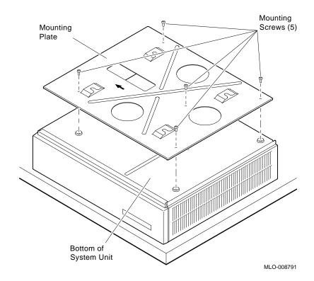
Position the System Unit on the Edge of the Desktop Keeping the system unit upside-down, position the unit so that it extends no more than 10 centimeters (4 inches) over the edge of the desktop as shown in Figure 3.
