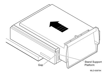
With the unit attached to the floor stand, lift the assembly into an upright position on its base as shown in Figure 6.
