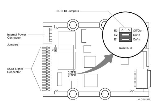
Figure 3–3 RZ5x Disk Drive SCSI ID Jumper Location
