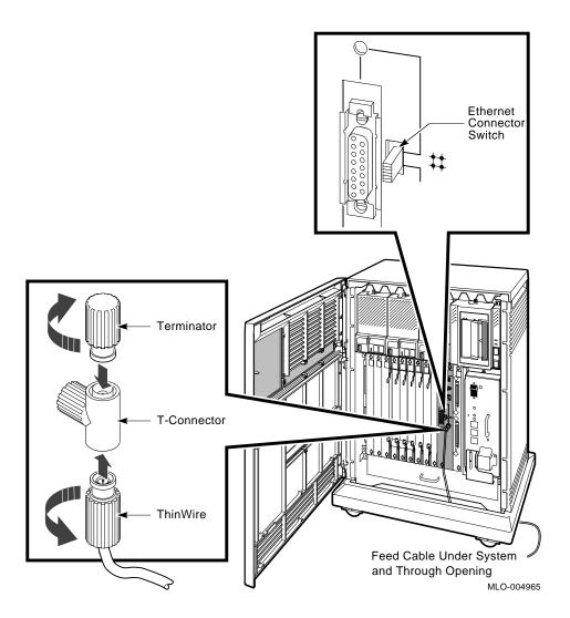
If your system requires one connection to the network, connect the ThinWire cable to the lower end of the T-connector and connect a terminator to the other end of the T-connector. Push in and turn the connector or terminator clockwise until it locks in place.
