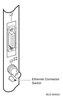
You can use the Ethernet Connector switch to select a ThinWire or a standard Ethernet connector.
