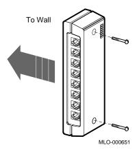
**NOTE:** Be sure you mount the cable concentrator less than 7.6 meters (25 feet) from the system, to ensure the BC16D cable reaches the system.
