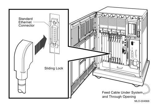
Make a standard network connection at the DESQA module as follows.
