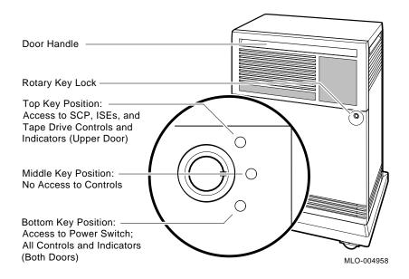
(SCP stands for System Control Panel and ISE stands for Integrated Storage Element.)
