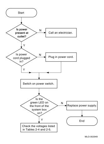
Figure 2-3 Flowchart for Troubleshooting the Power Supply
