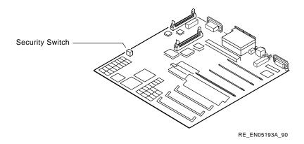
When you set the security switch on the system module to the insecure (down) position, the password is set to zero and the system is insecure.
