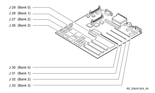
Insert the first MS44 memory module, with the side containing the bar code label facing up, into the connector on the system module. Gently press down on the module, until the tabs on the connector snap, locking the module into position.
