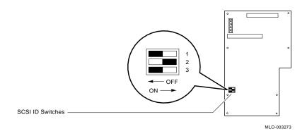
Table 3-6 shows the setting of the switches on the RX23 FDI board for the valid SCSI ID numbers.
