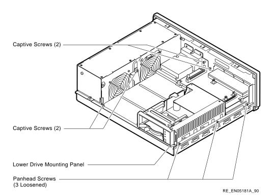
Figure 3-9 Releasing the Lower Drive Mounting Panel
