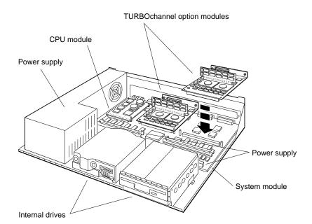
Figure 1-9 Inside the System Unit
