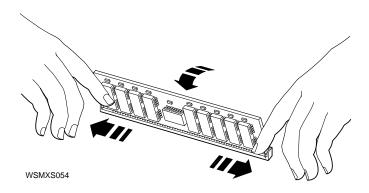
6. Tilt the memory module toward the front of the system unit until you can lift it out of the slot connector.
