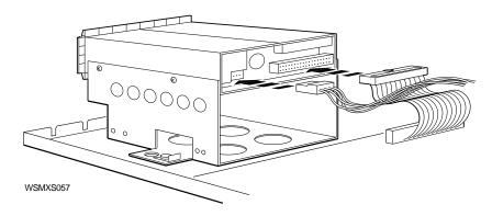
7. Stand facing the front of the system unit. The space for the drive is in the right front corner. Fit the tabs on the left side of the mounting bracket into the slots in the base of the system unit.
