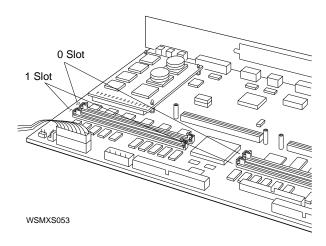
Figure 10-4 Inserting a Memory Module
