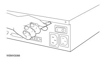
5. Pressing down on the two black leverage buttons on the back of the system unit and at the same time pressing up against the cover's edge, as shown in Figure 1–8, lift the back end of the cover about 6 inches.
