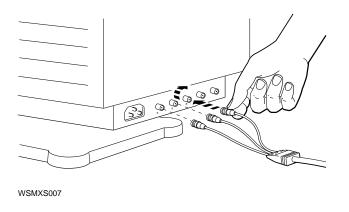
Figure 1-11 Connecting the Video Cable to the VRM17 Monitor
