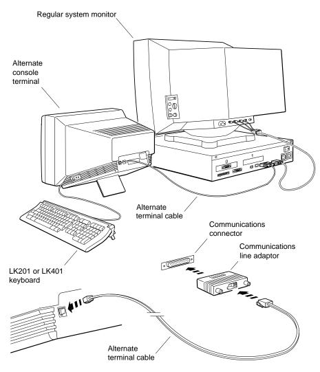
Figure 8-1 Installing a Console Terminal
