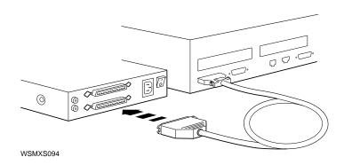
5. If this is the only expansion box you're connecting, place a terminator on the unused expansion box SCSI connector. Use the terminator that came with the expansion box.
