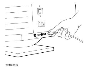
3. Connect the other end of the monitor video cable to the video connector on the back of the system unit (Figure 1-12).
