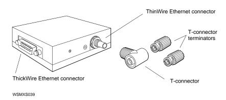
9. Notice that the ribbed part of the T-connector can be twisted from side to side. Press this ribbed part onto the ThinWire connector on the adapter and turn it to the right until it slides forward and locks into place.
