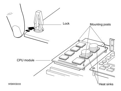
7. Keeping your hands well away from the heat sinks, grip the edges of the module and lift it up until it moves out of the connector on the base module. You may need to rock the CPU module from side to side very gently to loosen it.
