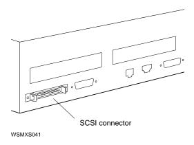
The system unit also has an internal SCSI connector to which the internal hard disk drive is connected. (The internal floppy disk drive is not a SCSI device.) For more information about connecting internal drives, see Chapter 9, "Internal Storage Devices."
