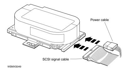
7. Stand facing the front of the system unit. The space for the hard disk drive is at the front of the unit, in the center. Fit the tabs on the left side of the mounting bracket into the slots in the base of the system unit.
