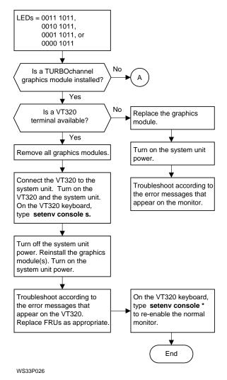
Figure 2-7 When the LED display is 0011 1011, 0010 1011, 0001 1011, or 0000 1011, 1 of 2
