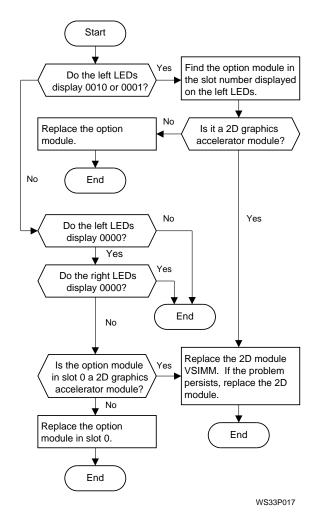
Figure 2-6 When the LED display is 0010 0011, 0001 0011, 0000 0011, or 0000 0000
