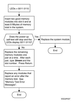
Figure 2-5 When the LED display is 0011 0110
