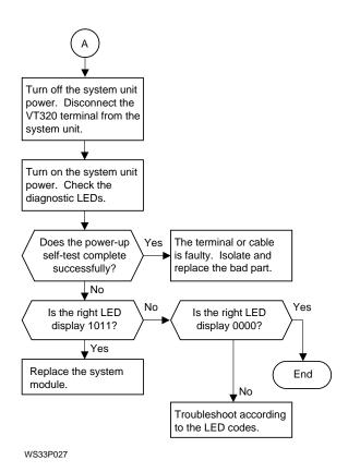
Figure 2-8 When the LED display is 0011 1011, 0010 1011, 0001 1011, or 0000 1011, 2 of 2
