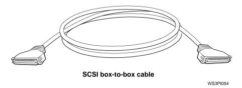
Attach one end of a SCSI box-to-box cable to the unused SCSI connector on the previously-installed box.
