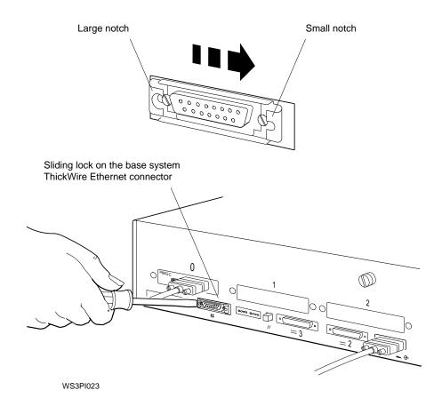
2. Find the ThickWire cable that you ordered for your workstation. Notice that one end of the cable has a sliding lock on it and the other does not.
