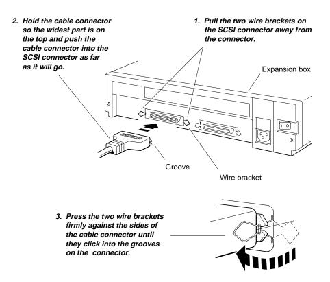
9. Connect additional expansion boxes to the first box (up to a total of three per system unit SCSI connector), using box-to-box SCSI cables.
