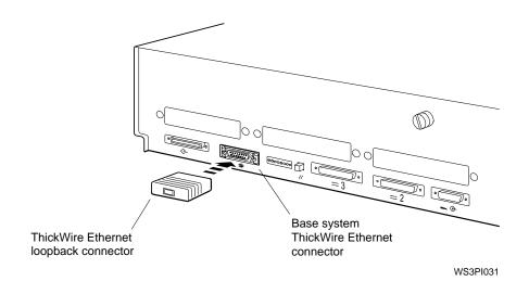
4. Put Ethernet loopback connectors on any other unused Ethernet connectors you may have in the TURBOchannel option slots. (Only one Ethernet loopback connector comes with your workstation. Extra connectors must be ordered separately.) Attach a SCSI controller terminator to the base system SCSI connector.
