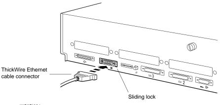
4. To lock the sliding lock on the base system Ethernet connector, push the protruding edge of the lock towards the center of the connector (using a flat-blade screwdriver) until it clicks into place. Check to make sure the cable is locked securely in place before proceeding.
