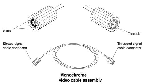
1. Attach the slotted cable connector to the monitor video connector.
