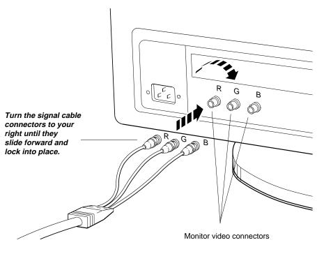
2. Connect the 3-pin cable connector to the workstation video connector in the system unit or TCE box.
