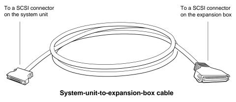
7. Attach the smaller connector on the system-unit-toexpansion-box cable to the SCSI connector on the system unit.
