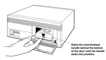
5. With the arrow on the tape cartridge pointing away from you, load the tape cartridge into the drive. (The owner's manual for the drive explains how to insert and remove tapes.)
