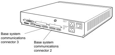
To connect a device with a 25-pin connector
