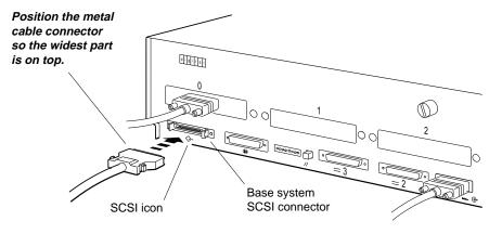
8. Attach the larger connector on the system-unit-toexpansion-box cable to one of the SCSI connectors on an expansion box.
