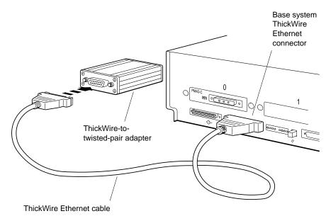
4. To lock the sliding lock on the cable connector, push the protruding edge of the lock towards the center of the connector until it clicks into place. Check to make sure the cable is locked securely in place before proceeding.
