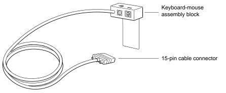
2. Plug the 15-pin connector on the keyboard-mouse cable assembly into the keyboard-mouse connector on the system unit.
