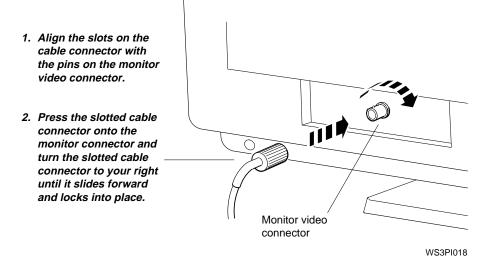
2. Attach the threaded cable connector to the video connector in the system unit or TCE box.
