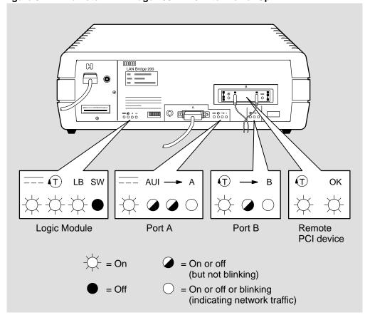
Figure 3-2: Remote LAN Bridge 200 LEDs After Power Up
