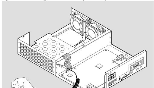
Figure 2–1: Attaching the ESD Grounding Wrist Strap
