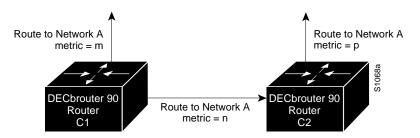
Figure 6–3 Determining IGRP Path Feasibility
