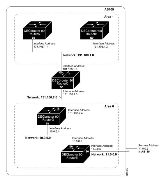
Figure 6–16 Sample OSPF Autonomous System Network Map
