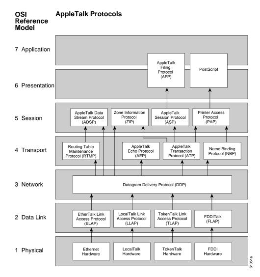
Figure 2–2 AppleTalk and the OSI Reference Model
