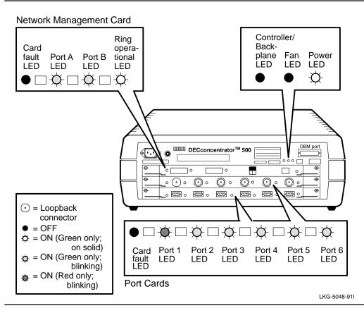
2. Remove the loopback connector. The port LED blinks green again.
