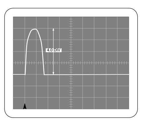
Figure B–1: TDR Pulse Display – Ideal Termination
