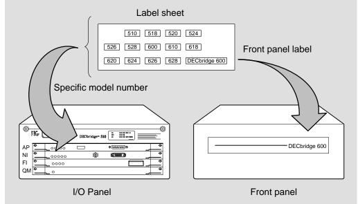
Figure 2–5: Locations for Applying Upgrade Labels
