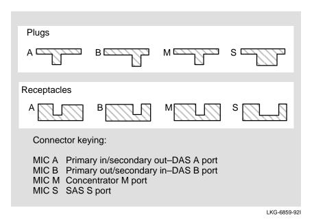
The position of the keyway on the MIC plug determines the type of receptacle to which it connects. A MIC S plug fits all receptacles. The other MIC plugs and receptacles (type A and B) must match for proper installation.
