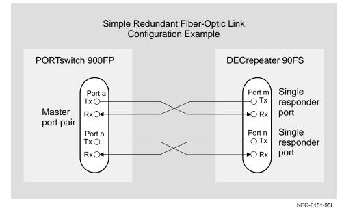
Once these ports are properly configured using HUBwatch and connected together, one connection is the active link and the other is the standby link.
