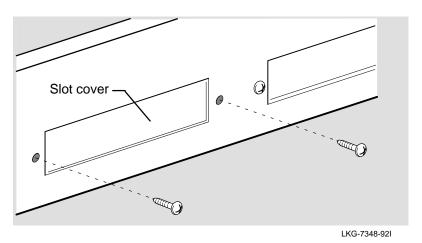
2.3 Installing the Controller
