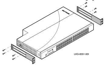
2 Position and secure the single-slot hub unit in the equipment rack.
