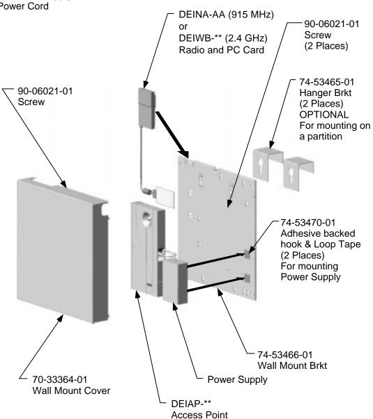
Mounting procedure for DEIAP-WM (RoamAbout Wall Mount Kit) For use with DEINA-AA or DEIWB-\*\* Indoor Radio and Antenna
