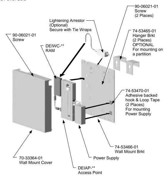
Mounting procedure for DEIAP-WM (RoamAbout Wall Mount Kit) For use with indoor omni directional antenna included with DEIWC-\*\* or the outdoor antenna purchased separately.
