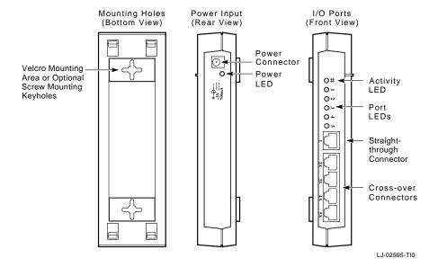
Figure 1–2 Digital Ethernet Multiport Office Network Repeater Wiring Configuration
