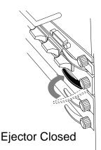
**5** Tighten the black captive screws on the module.
