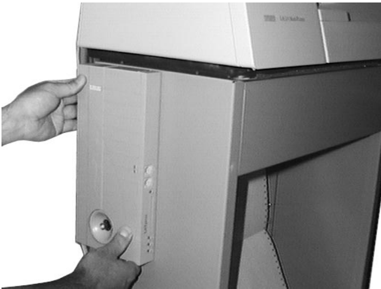
Figure 1-9 Attaching LATprint ThinWire Ethernet Interface to the LA424
