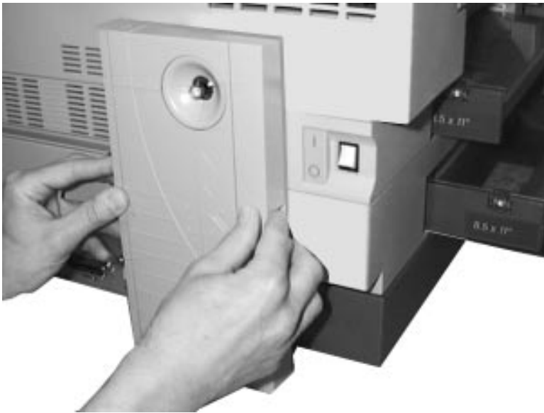
Figure 1-7 Attaching LATprint ThinWire Ethernet Interface to the DEClaser 3200
