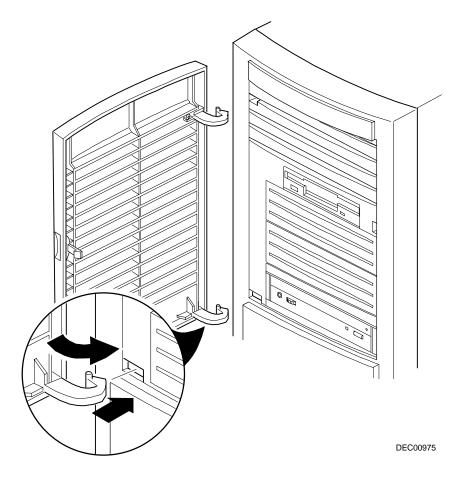
Figure 1-14. Replacing the Front Bezel Door
