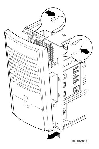
Figure 6-1. Removing the Front Bezel
