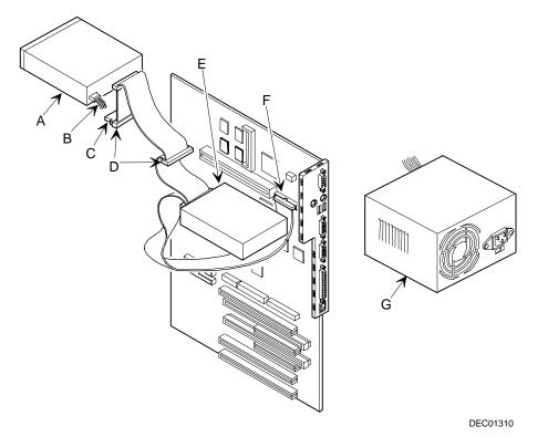
Figure 6-9. SCSI Device Data Cable Connections
