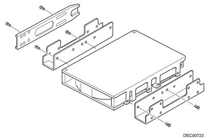
Figure 6-2. Installing Drive Rail and 31/2-Inch Device Brackets
