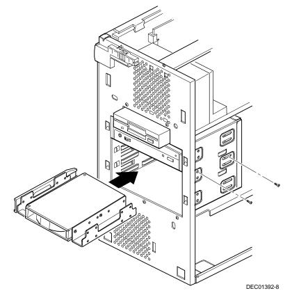
Figure 6-3. Installing a 3<sup>1</sup>/<sub>2</sub>-Inch Device
