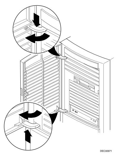
Figure 1-13. Removing the Front Bezel Door
