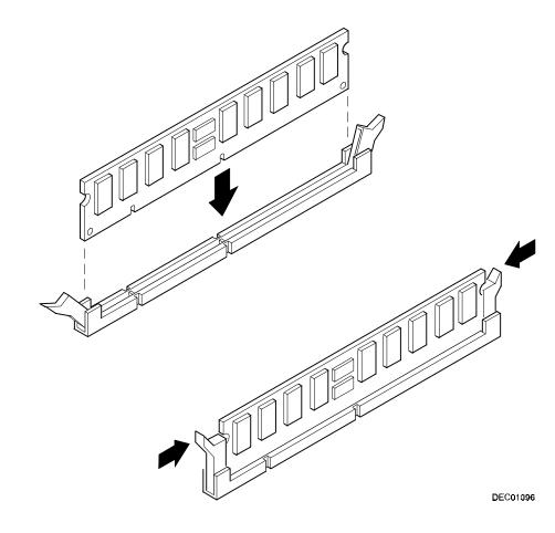
Figure 4-2. Installing a DIMM
