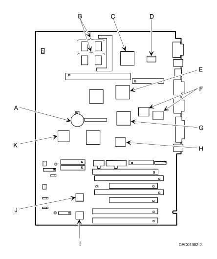
Figure 3-2. Main Logic Board Components
