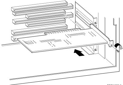
Figure 5-3. Installing an Expansion Board
