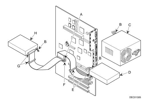
Figure 6-8. IDE Device Data Cable Connections
