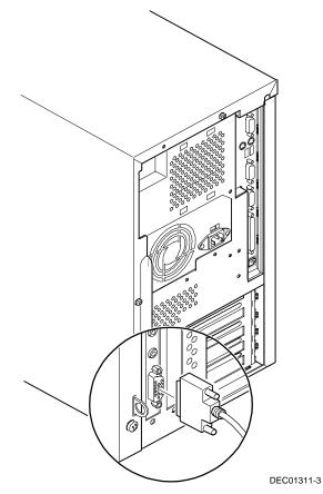
Figure 1-9. Connecting a MIDI/Joystick Device
