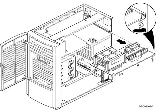
4. Push out on the two plastic ejectors to release the Pentium<sup>®</sup> II processor module from the main logic board.
