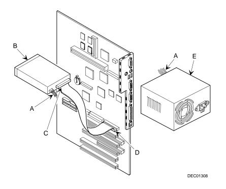
Figure 6-7. Diskette Device Data Cable Connections
