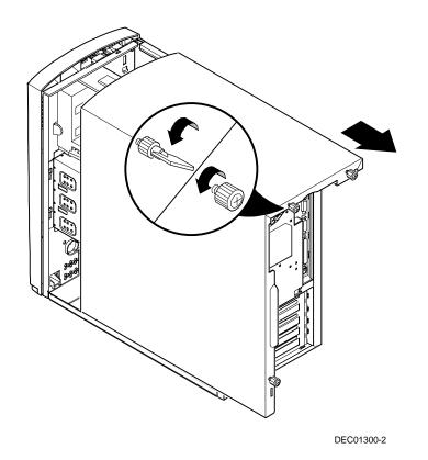
Figure 1-3. Removing the Outside Cover
