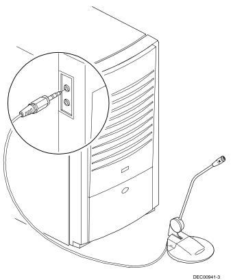
Figure 1-8. Connecting a Microphone
