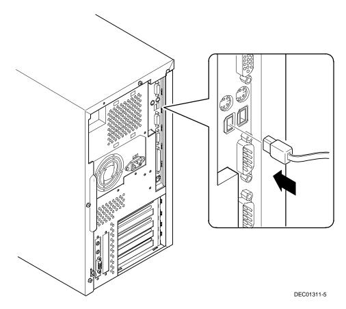
Figure 1-11. Connecting a USB Device
