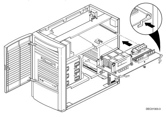
Figure 3-13. Replacing the Pentium<sup>®</sup> II Processor Module
