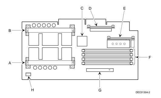
Figure 3-5. Pentium<sup>®</sup> II Processor Module Component Locations
