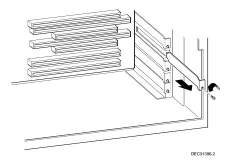
Figure 5-2. Removing a Metal Filler Plate
