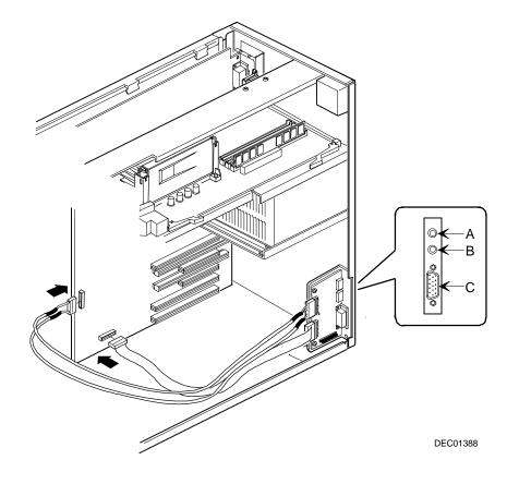
Figure 3-6. Audio/MIDI/Joystick Adapter Card Connectors
