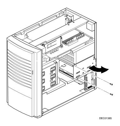
Figure 6-5. Accessing the Internal 3<sup>1</sup>/<sub>2</sub>-Inch Device Bay
