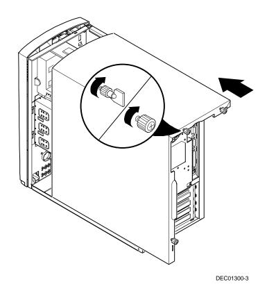
Figure 1-5. Replacing the Outside Cover
