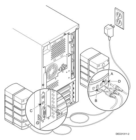
Figure 1-6. Connecting Speakers
