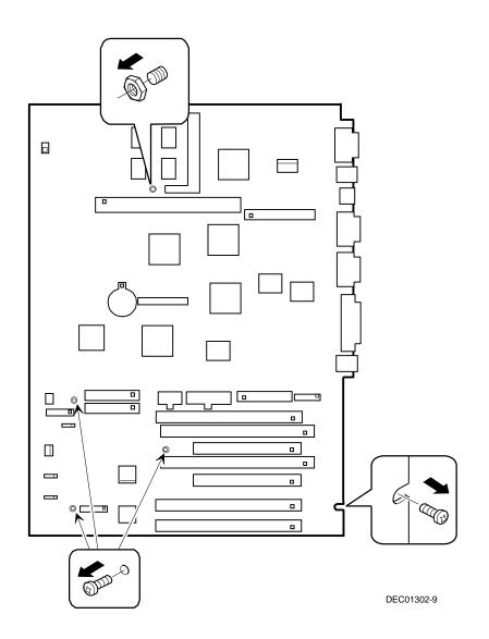
Figure 3-7. Removing the Main Logic Board
