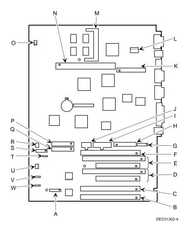
Figure 3-4. Main Logic Board Connectors
