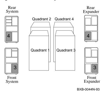
Figure 1-3 Cabinet Battery PIU Placement
