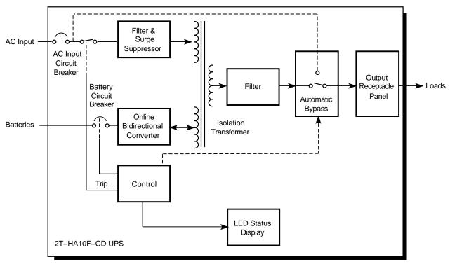
Figure 1–1 2T-HA10F-CD UPS Functional Diagram
