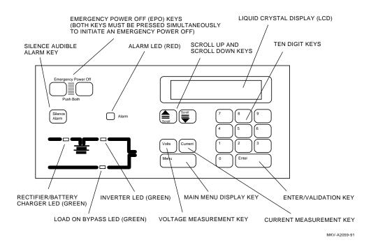
Figure 2–1 System Status and Control Panel (SS&CP)
