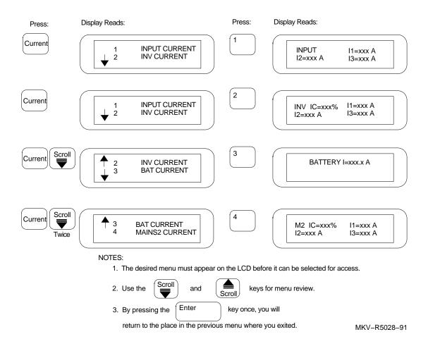
Figure 2–3 Current Measurements
