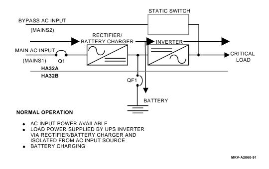
Figure 2–5 Normal Operation Power Flow
