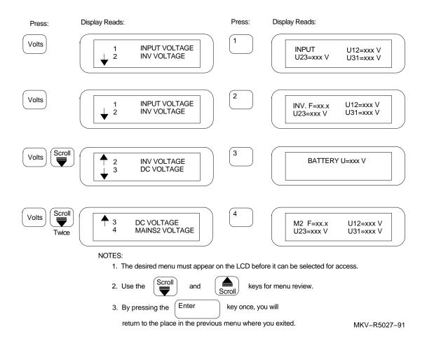
Figure 2–2 Voltage Measurements
