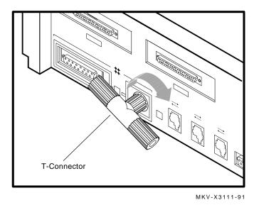
4. Connect the loopback connector to the standard Ethernet port on the back of the system unit. If needed, rotate the T-connector slightly to make room for the loopback connector.
