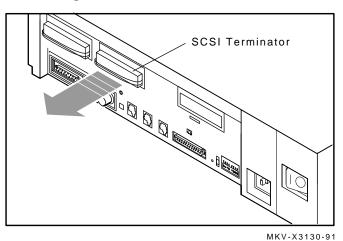
Figure 3–1 Removing SCSI Terminator
