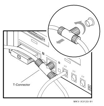
7. Check that you have not disconnected a terminator from an active ThinWire segment. This would disrupt network operation.
