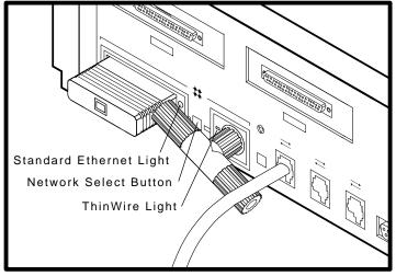
Figure 4–1 Position of Network Select Button and Ethernet Lights
