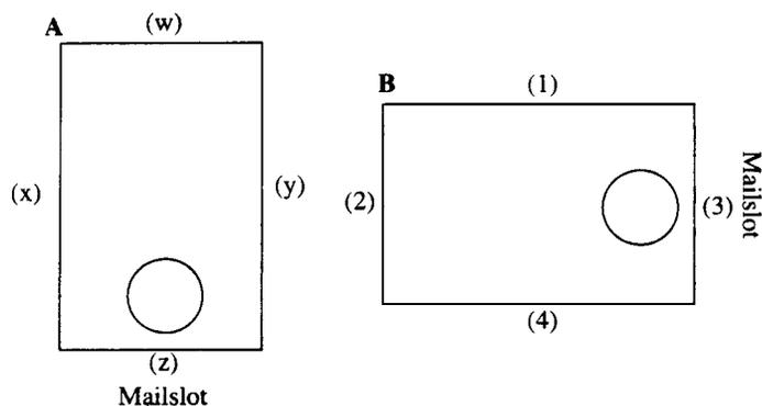
**"A" orientation - usually in a row of peripheral cabinets.**
