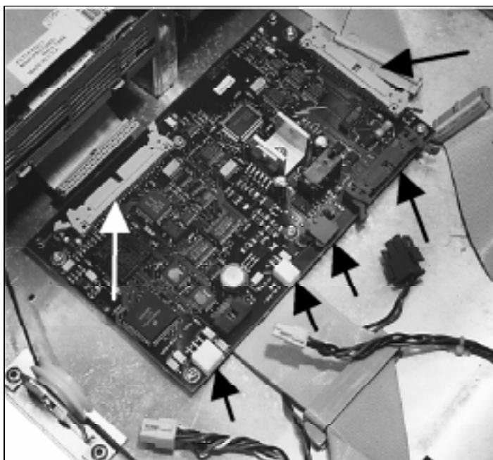
5. After replacing the Controller PCA, re-initialize the NVRAM by executing tests “*SET DEFAULTS*” & “*CLEAR ODOMETERS*”. Reference section “*Re-initializing the Jukebox Controller PCA After Service*”.
