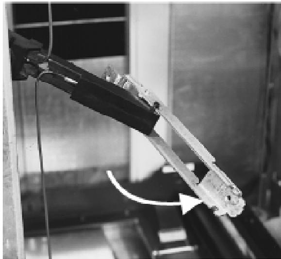
4. Release the tension on the rear rope tensioner (drive rope). Grip the rope tensioner plastic section with one hand and pull back the metal section with your other hand to release the metal securing tab seated in the plastic section. The metal section will swing out and off pivoting pegs on the plastic section.
