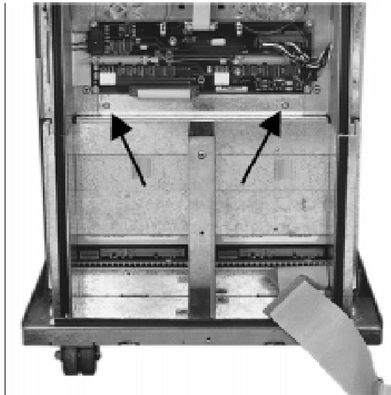
Figure 5–14 Optical Drive Mounting
