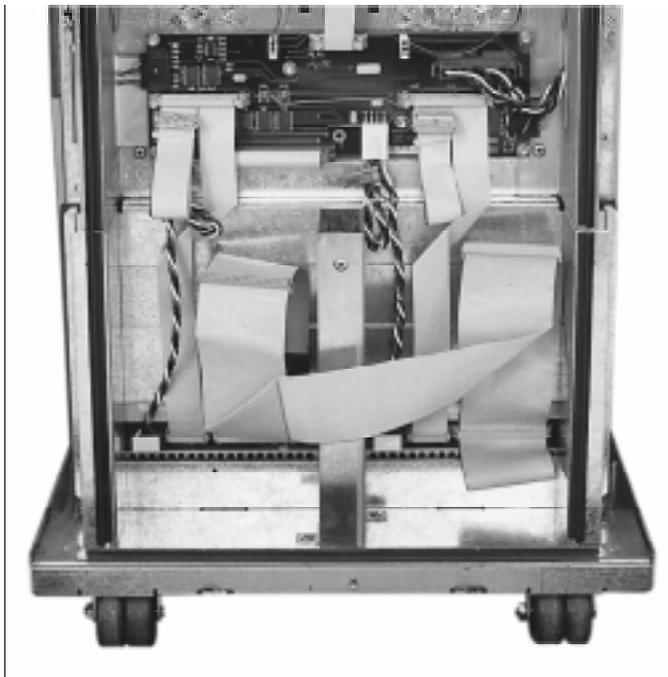
3. Remove the RFI panel covering the drives. Remove the two T-20 screws from the top of the RFI panel. Tip the panel out and up. The panel is held at the bottom by positioning tabs. As you pull the RFI panel up and away, help the SCSI cable thread through its hole in the panel.
