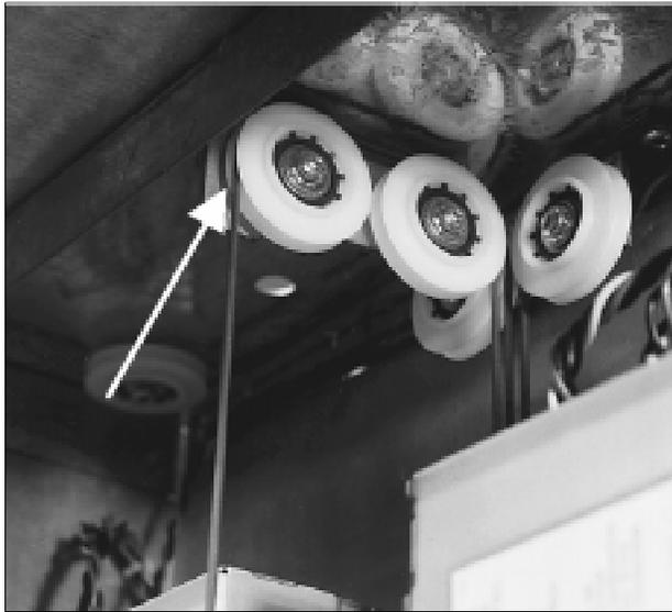
**Figure 5-37 Disconnecting the Drive Rope From a Tensioner**
