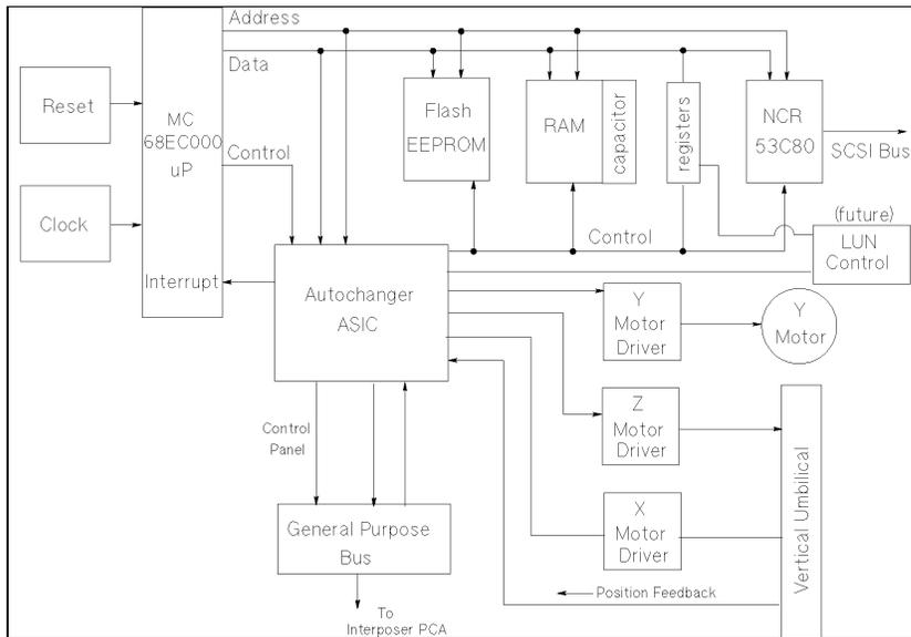
The MICROPROCESSOR is a Motorola MC68EC000 running at 12.288 MHz. This microprocessor controls all processes on the controller PCA such as servos, SCSI interface, and commands to the control panel.
