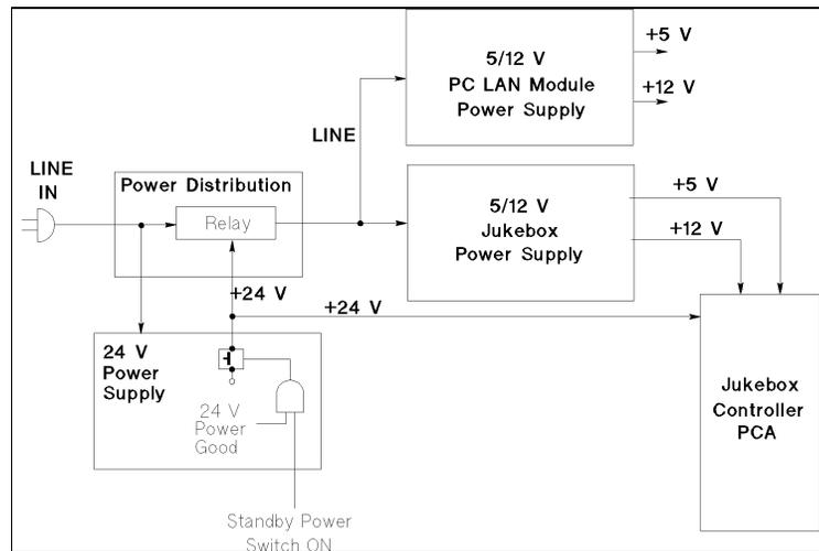
Line power is connected through the power distribution PCA in the interface (or LAN module) enclosure. Connection is direct to the 24-volt power supply.
