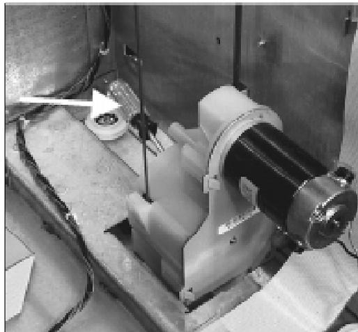
5. Remove the T-10 sheet metal screw that holds that holds the capture spring down.
