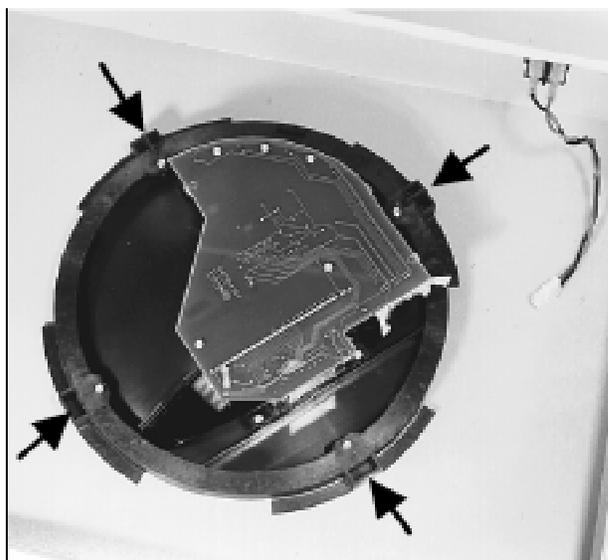
3. Remove the four T-10 sheet metal screws from the control PCA retaining ring. This detaches the control panel PCA from the mounting assembly on the panel.
