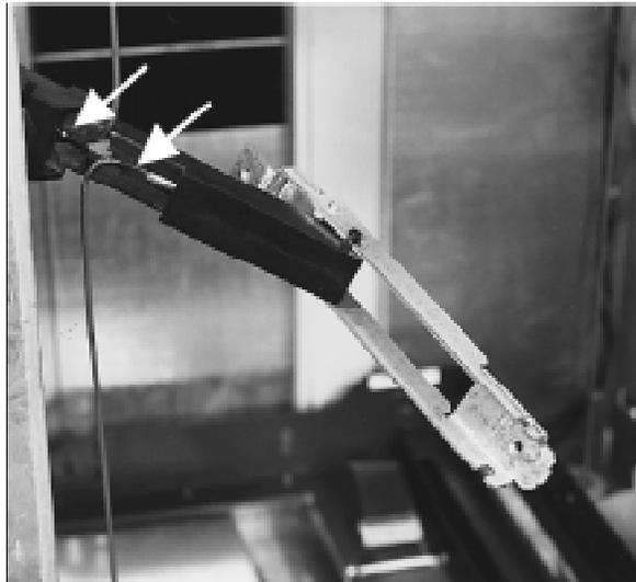
**Figure 5–39 Disconnecting the 3-Rope Coupler**
