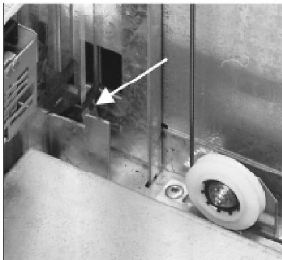
3. Remove the encoder strip anchor. Remove the T- 15 screw located on the top front edge of the unit.
