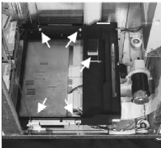
7. Disconnect the umbilical cable on the underside of the frame. Do this before moving the translate frame down to the bottom of the jukebox in the next step.
