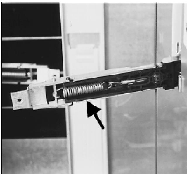
9. Remove the first two ropes from the rope coupler. The center (second) rope is the drive rope. It is not necessary to remove the rope coupler completely.
