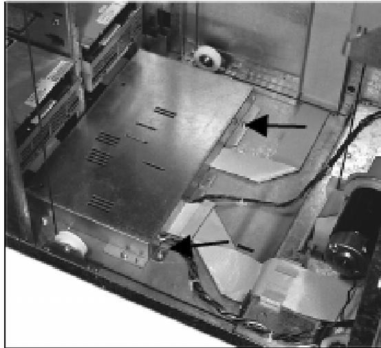
3. Disconnect the following cables from the controller PCA: SCSI cable, Power cable, Motor encoder and power cables, Picker cable.
