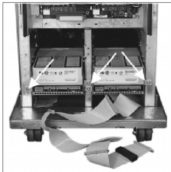
5. Slide the drive out along its positioning tabs.
