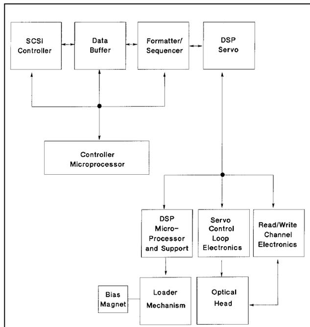
There are four major sub-assemblies within the optical drive: the controller PCA, servo PCA, loader mechanism, and the optical head.
