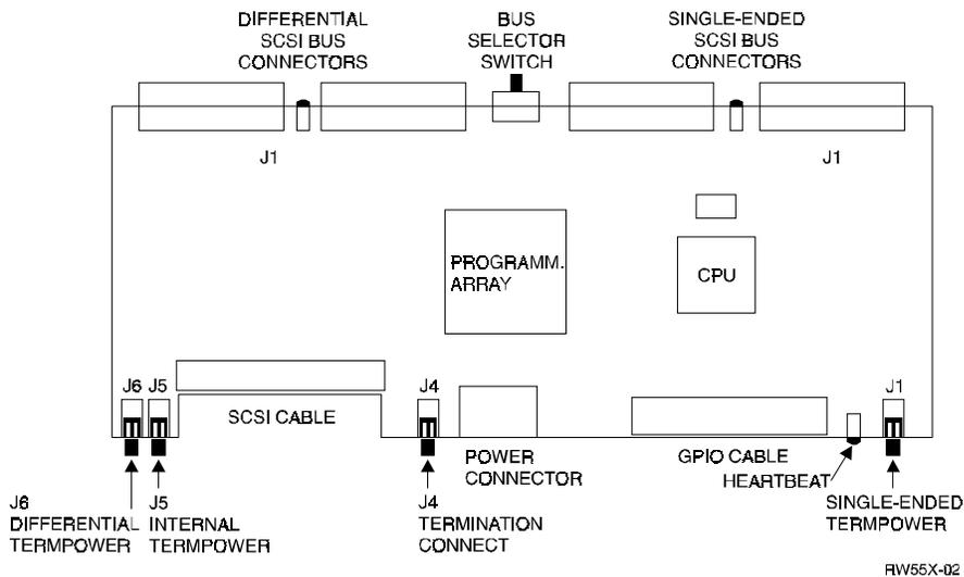
The two large components on the PCA are the Field-Programmable Gate Array and the microprocessor. The microprocessor is an 80C52 that has flash-programmable memory on board. (There are no boot ROMs on this PCA). The chip can be programmed, however it must be disconnected from the PCA to do so. The Field-Programmable Gate Array can not be programmed.
