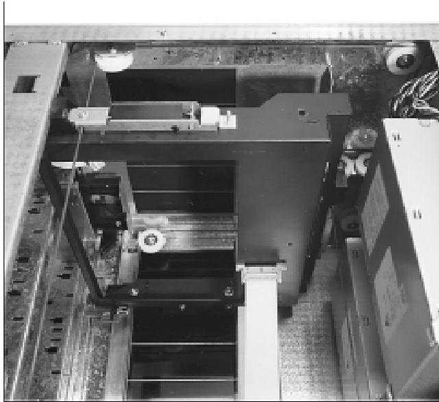
3. Raise the translate frame up to the top of the jukebox and secure with a screwdriver placed in the vertical motor gear box securing hole.
