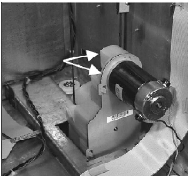
3. Remove two T-15 motor mounting screws on the gear box.
