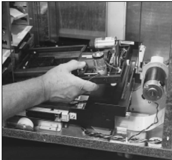
9. Remove whatever tool is being used in the vertical motor gear box.
