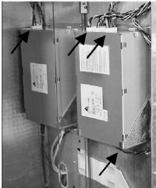
2. Remove the power plug from the bottom of the supply.
