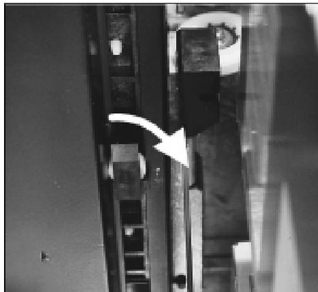
**Figure 5-23 Rotating the Picker Assembly Out of the Translate Frame**
