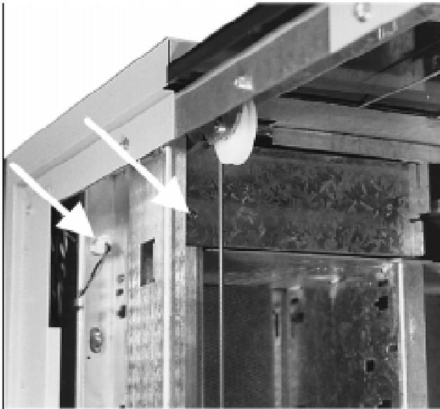
3. Remove the T-20 screw that holds the control panel access plate. The right side of the baffle is held by a tab fitting into a slot in the mailslot housing. To remove, rotate the left side of the panel back and away.
