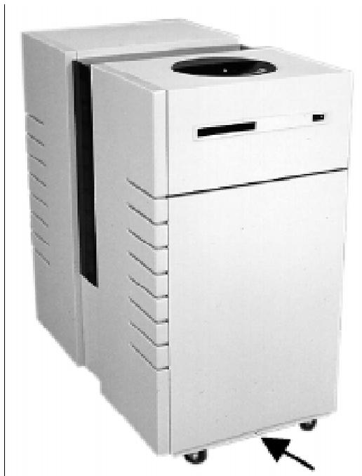
1. Switch off the power to the jukebox by placing the power standby switch to OFF (0) on the right side.
