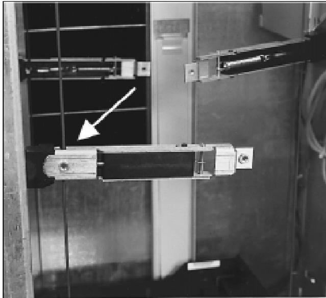
**Figure 5–35 Pivoting The Tensioner Lever To Release Tension**
