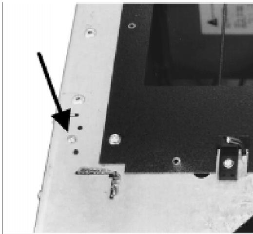
**Figure 5–32 Top Mount Of Encoder Strip**
