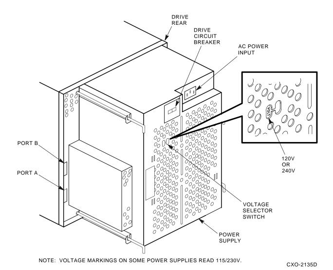
Figure 2-5 Drive Voltage Selector Switch
