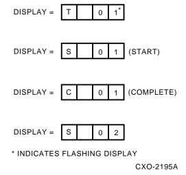
Figure 3–3 OCP Displays During Normal Testing
