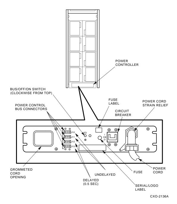
Figure 2–2 881 Power Controller (Example)
