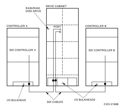
Figure 1-3 RA90/RA92 Dual-Port Configuration
