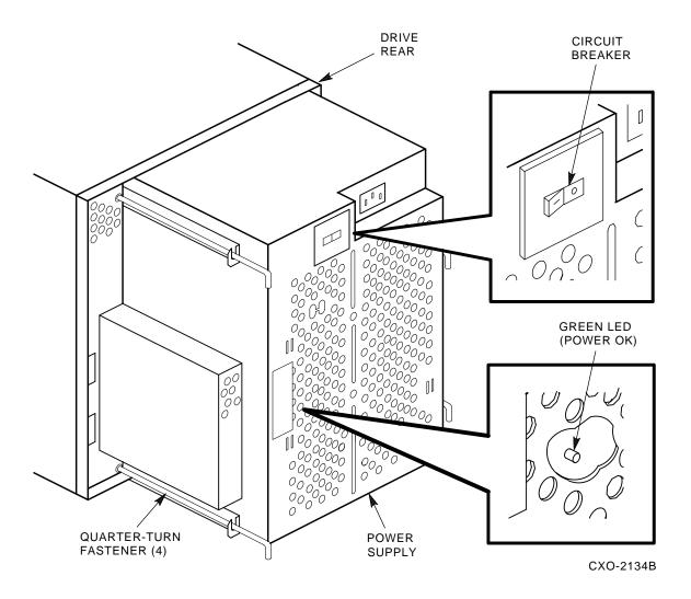
Figure 2-4 Drive Circuit Breaker Location
