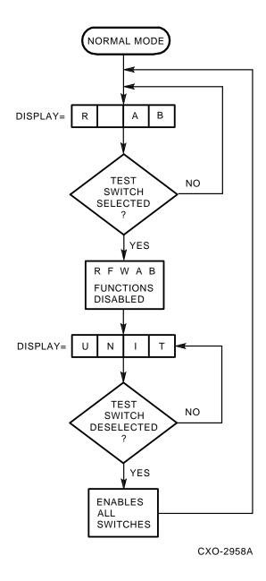
Figure 3-5 Alternate Unit Address Display Mode Flowchart
