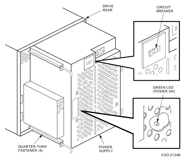
Figure 3-2 **Power Supply Indicator**
