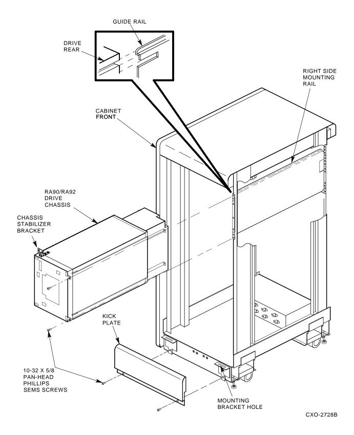
Figure 2-4 Cabinet Rails and Kick Plate (Front)
