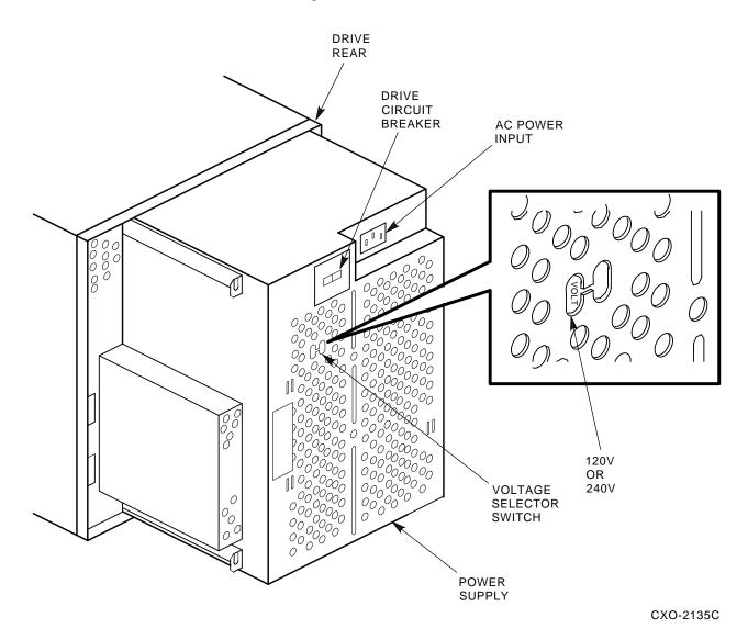
Figure 2-7 RA90/RA92 Voltage Selector Switch/Circuit Breaker
