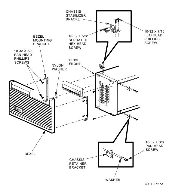
Figure 2-1 Installing Disk Drive/Cabinet Hardware, Front View
