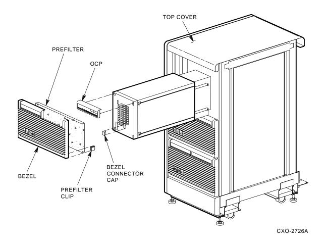
Figure 2-3 Removing Bezel, OCP, Bezel Connector Cap
