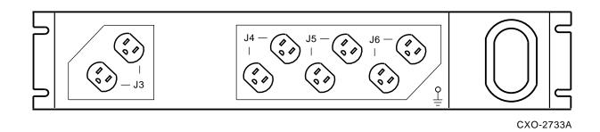
Figure 3–3 874 Power Controller, Rear View
