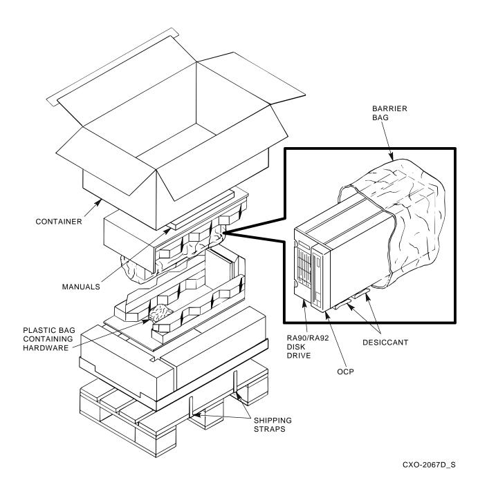
Figure 1–2 RA90–NA/RA92–NA Add-On Shipping Container Contents
