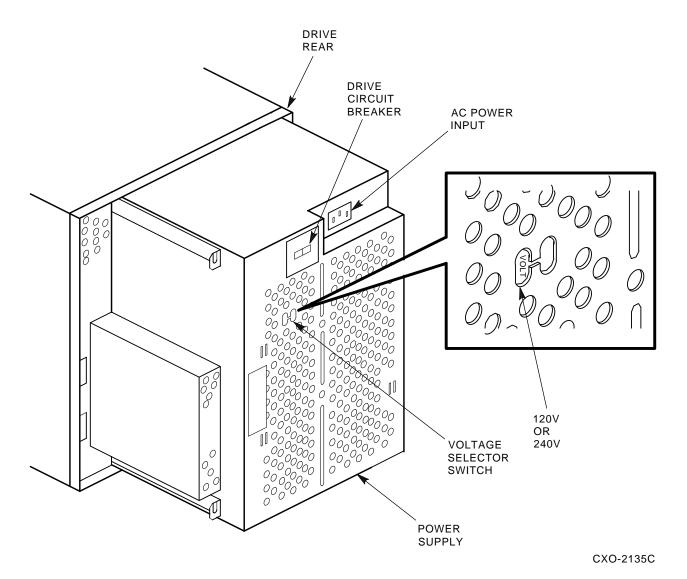
Figure 3–4 RA90/RA92 Voltage Selector Switch/Circuit Breaker
