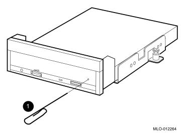
**1** Paper Clip—Insert the clip 35 mm into the emergency eject hole.
